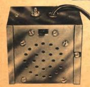
A highly efficient Geiger Counter Transistorized Amplifier Circuit for speaker operation. This Transistor Geiger Amplifier will make your Geiger Counter clearly audible through a speaker with volume to spare. Just plug it into the Geiger Counter!
