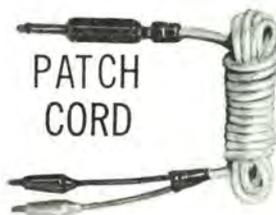
A 6 foot two-conductor cord with plastic insulation and re-enforcements at stress points. Has phono plug on one end which fits into an adapter with standard phone plug. The other end has two insulated color coded alligator clips. Use to take sound from a speaker to feed a tape machine, to connect to mike output, connect amplifier, phono, etc., etc.
