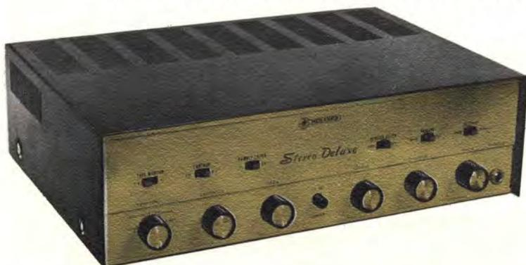
All of the latest engineering features combined in one compact unit to deliver clean amplification of fine sound. Delivers 30 watts of music power per channel for a 60 watt total. Response from 20 to 50,000 cps  $\pm$ 0.5 db.; with a 9 tube-2 diode, push-pull, fixed bias circuitry. Contained in a smart metal cabinet with brushed-gold face plate. 15 $\frac{3}{4}$ " wide, 5" high, 12 $\frac{1}{2}$ " deep.
