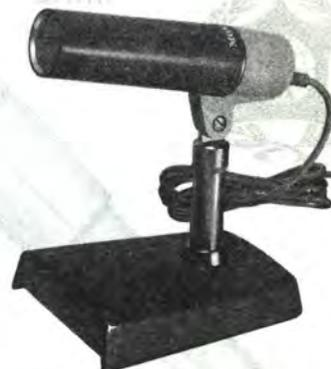
A big desk mike with barrel 5 1/4" x 1 1/4" on a sturdy desk stand 5 1/4" in height. Has low-range compensating barrel, special plastic diaphragm for high sensitivity and rich low ranges and excellent high frequency characteristics. All parts are the finest materials and carefully finished. Output impedance: 50 K Ohms, output level: -55db + 3 db at 50 K, response: 50 to 15,000 cps.
