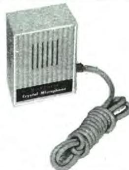
Tiny "Match-Box-Size" Crystal Microphone in an ivory plastic case only 1 5/8" x 2 3/8" x 1" deep. High Impedance. Response: 200 to 7,500 cps. Fitted with a 3 foot plastic covered cord.
