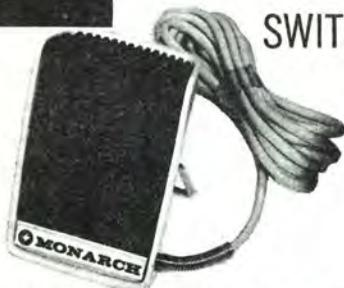
An exceptionally fine hand mike in a smart modern case of black and white plastic with a locking slide switch, 5 foot plastic covered cord, and flip-back metal stand for desk use. Measures 3" x 2 1/4" x 1". A built-in transformer minimizes induction and interference. Response: 200 to 10,000 cps, impedance 600-50K Ohms, sensitivity: -55db +3db at 50KΩ.
