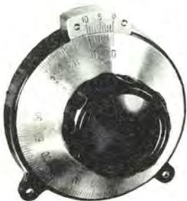
8:1 RATIO precision vernier dials with a heavy black bakelite base and nickel-silver dial plates with deeply etched, clearly legible scales. Moulded knob with fluted grip. Internal parts of phosphor bronze and brass for long-life dependability. Calibrated 0 to 100 in 180° rotation. For front panel mounting. Choice of four sizes.
