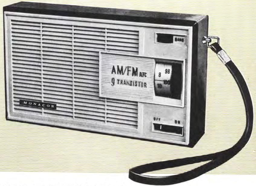
Hand-size unit in cleanline plastic case with distinctive gold escutcheon, vernier tuning dial, and convenient wrist cord. Features the most advanced nine-transistor circuitry, huge ferrite antenna, and special wide-range PM speaker. With AFC circuitry to assure the finest drift-free sound on both AM and FM bands. Modestly priced for the thrifty purchaser. Complete with battery and earphone, in a bright display carton.
