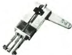
Stereo-monoaural turnover ceramic with response from 20 to 20,000 cps. Dual sapphire for 16, 33, 45, 78 rpm. Output: 20 mV.
