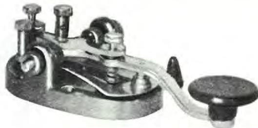
STANDARD PRECISION-BUILT TELEGRAPH KEY with smooth, velvet action for code practice and use with transmitters. Eight ball bearings supporting the key are completely adjustable for friction. Contacts are 1/8" pure silver and are also easily adjustable for contact spacing and tension. Heavy brass base is drilled for easy mounting.
