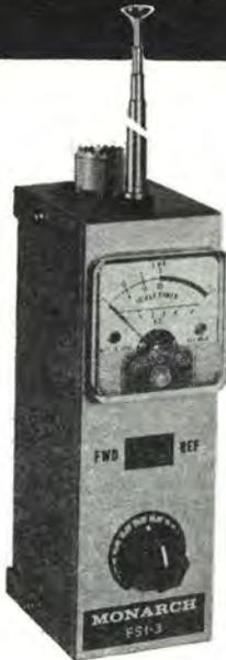
An excellent combination unit for either home station or mobile use... as an accurate Standing Wave Bridge and a sensitive Field Strength Meter. 52 Ohm impedance. Will take a full kilowatt and can remain in the line all of the time.
