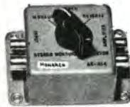
Simple, convenient switching from stereo to monaural to reverse. Has two phono jacks input and two phono jacks output. Dual channel feed-through for stereo. Outputs are connected for monaural use. shielded metal housing attractively finished, measuring 2" square and 1" deep with mounting flange
