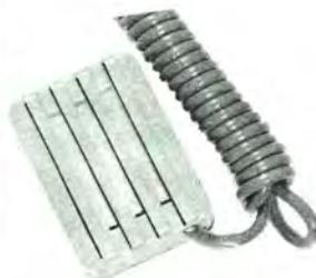
Non-directional mike in a clean-line plastic case only 1 3/4" x 1 1/4" x 9/16". 100 to 9,000 cps; -50 db sensitivity. With strong spring clasp for attaching to lapel or shirt front and 5 foot shielded cord.
