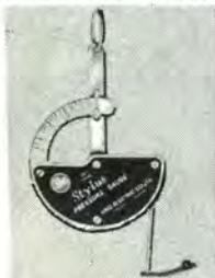
Operates on simple lever principle. Unaffected by heat, humidity, etc. Permits accurate measurement with arm in normal playing position. 0 to 30 gram scale. Heavy gauge aluminum alloy **NO. SPG-1**
