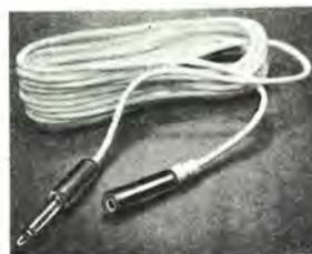
A durable 25 foot extension cord for use with stereo earphones. Monarch Model ES-300 or many others in the field. Plastic covered 3-conductor cable with 3-circuit standard phone plug and 3-circuit barrel jack.
