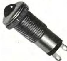
Precision built, only 1" in length, requires 5/16" mtg hole. For 115 v lines use 2 100K ohm resistors in parallel- for 230v lines, 250K resistors in parallel. Choice of red, yellow or clear lens. Pls specify choice.
