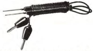
With rubber capped special alligator clips and extra long prods. The alligator clips have special nose to fit directly into standard Banana Jacks. Plastic test prod handles 3 1/2" long, 3/8" diameter. 48" plastic red and black leads.
