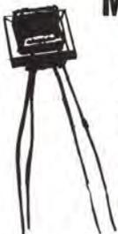
These tiny transformers use finest quality cores, made of hydrogen heat processed permalloy. Fine coil wire of 0.025 mm diameter is used. A special type of vacuum impregnated insulation is employed, making these transformers impervious to corrosion and coil wire breakage.
