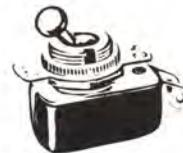
S. P. S. T. Toggle Switch 1/2" Shank, Ball Handle, Molded Bakelite Case, with "on-off" plate. Rated 3 amps, 250 Volts, 6 amps, 125 Volts. U.L. Approved. Supplied with two Mounting Nuts.
