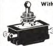
Manufactured by H. & H. for Philmore. UL Approved. Ball handle, molded bakelite case, 3/8" shank, rated 3 amp, 250 volts, 6 amp, 125 volts. Supplied with two mounting nuts.
