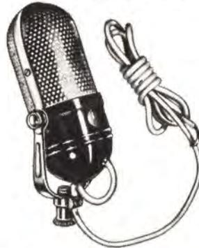
Omni-directional studio type crystal microphone, suitable for conference groups, PA, tape recordings, etc. Dual phased crystal units, vertically mounted. Mounting thread 5/8"-27. Supplied with 4 feet plastic covered microphone cable.
