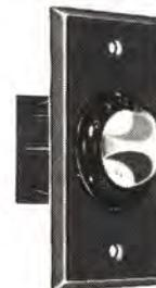
Selects any combination of three separate Hi-Fi speaker systems. Selects speakers 1, 2, or 3 separately, or 1 and 2, 2 and 3, 1 and 3, or all three together. Screw terminals are marked for amplifier and speaker connections. Supplied pre-mounted on brass wall plate to fit into standard wall switch box.
