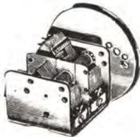
Superheterodyne, with trimmers, compact size. Standard curve. Ball-bearing. Lo-loss insulation. firmly staked, aluminum rotor and stator plates. Height  $1\frac{5}{8}$ " x depth  $2\frac{1}{4}$ " x width  $1\frac{3}{8}$ ". With  $2\frac{1}{4}$ " Dial Pulley. Clockwise rotation.
