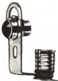
Mounts in  $\frac{5}{16}$ " diameter hole. Nickel plated, overall height  $1\frac{7}{8}$ ", depth behind panel  $1\frac{1}{8}$ ", takes standard miniature base pilot light. Smooth faced jewel, available in red or green. Specify color. No. 565. List, each \$ .31
