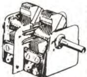
T.R.F. COMPACT SIZE Standard curve. Ball bearing. Lo-loss insulation. Firmly staked aluminum rotor and stator plates. Height  $1\frac{3}{8}$ " x depth  $2\frac{1}{4}$ " x width  $1\frac{3}{8}$ ". Counter-clockwise rotation. Complete with trimmers. Shaft length  $1$ " x  $\frac{1}{4}$ " diameter.
