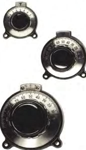
Smooth friction vernier drive dials, with clearly etched numerals on professional-finish satin background. Calibrated over 180° reading from 0 to maximum setting by clockwise rotation. Planetary drive with 8 to 1 ratio. Precision brass and bronze parts are mounted in attractive black phenolic housing. Furnished with matching black phenolic knob. Surface mounting for ¼" shaft.
