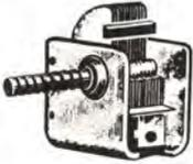
Shaft length  $1\frac{1}{2}$ " x  $\frac{1}{4}$ " dia. Aluminum rotor and stator plates firmly staked. Lo-loss bakelite insulation. Improved ball bearing. Height  $1\frac{1}{2}$ " x depth  $1\frac{5}{16}$ " x width  $1\frac{1}{8}$ ". Counter-clockwise rotation. Compact size.
