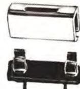
Single fuse mounting base for 3AG fuses, with removable slide-on metal shield cover. Top chassis single hole mount. 1/8" thickness, molded bakelite base.
