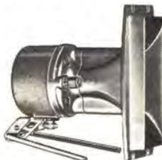
Dual mounting — either externally on stand supplied with unit, or internally into a speaker system. Aluminum wound voice coil 8 ohm impedance. Will handle up to 20 watts. Exceptionally smooth speaker response from 1700 to 16000 CPS.
