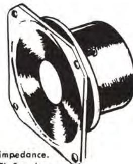
1 1/2" Diameter x 15/16" deep. Finest loudspeaker made, affords high quality sound! The magnet weighs .5 oz., is made of Alnico V, and is mounted in a speaker pot cover. The speaker is adaptable to either 8 ohm or 3.2 ohm voice coil impedance. Can also be used as a tweeter for Hi-Fi Speaker systems.
