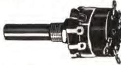
For miniaturized transistor and tube circuit construction. All controls have audio (semi-log) taper. Mounts in 5/16" hole in panels up to 1/4" thick. Have 1/4" flatted shafts x 3/4" long. Supplied complete with mounting nut and washers. Body diameter 3/4" x 9/16" deep. Individually boxed.
