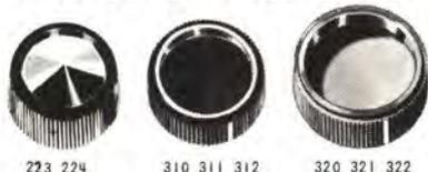
Modern styling for Hi-Fi and Radio applications. Non-slip gripping surface. All knobs have molded-in brass inserts for  $\frac{1}{4}$ " shaft. Supplied with set screw.
