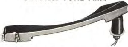
Exceptionally light-weight tone arm and crystal cartridge that can be used for stereo or monaural recordings at the flick of the wrist. The specifications of the cartridge are the same as our No. PC75STL cartridge. The frequency response is 40-13000 CPS. Output 0.4 volts. Comes complete with mounting hardware. Includes two separate shielded cables and two sapphire needles. Individually boxed.
