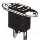
Suitable for accessory equipment power outlets on amplifiers, pre-amplifiers, clock radio chassis etc. 1 1/8" mounting centers. Requires a 3/4" x 3/8" rectangular cutout. U.L. approved.
