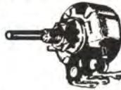
Extremely compact: overall dimensions, shaft 3/4", bushing 1/4", pot diameter 3/4", 1/2" thick. 1/4-32 bushing thread. 1/8" diameter shaft. Switch rated 1 amp at 125 V AC-DC.
