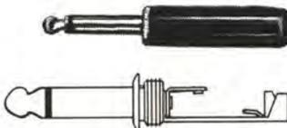
Solder lug type with cable clamp terminal. Similar to the PL55 plug, except without screws. Supplied with Red or Black bakelite barrel. All parts nickel plated. Fits all standard type Jacks.
