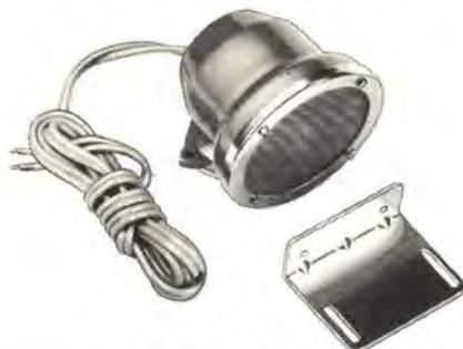
Handles up to 20 watts of audio power, with frequency range 3000 to 17000 CPS. Built-in crossover network. Mounting bracket with 2 mounting holes is attached. Metallic grey finish housing. 3-ft. twin rubber covered cord is included. Extra vertical, adjustable bracket suitable for flush mounting against baffle supplied complete with hardware. Voice coil impedance 16 ohms. Size 2 3/4" dia. x 2 1/4" deep. Individually boxed.
