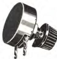
Used to control volume of rear seat auto speakers with tube or transistor radios, or any small speaker of 4, 8 or 16 ohm impedance. Supplied with protective back cover, knob, hex nut and washers. Diameter of control 1 1/8". 3/8" threaded bushing x 1/4" long. Shaft length 1/2" x 1/4" diameter.
