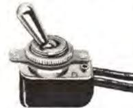
S.P.S.T. Toggle Switch. 3/8" Shank, Bat Handle. Molded Bakelite Case, with 2-6" Insulated leads and "on-off" plate. Rated 3 amps, 250 Volts, 6 amps, 125 Volts. U.L. Approved. Supplied with two Mounting Nuts.
