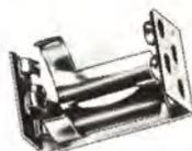
Designed to accommodate 4— $1\frac{1}{2}$  Volt standard Penlite Batteries. Sturdy construction. Has two mounting holes with  $2\frac{1}{2}$ " mounting centers. Specially designed for Transistor Radios and Model Airplanes. Also adaptable for many other uses. Batteries can be connected in series or paralleled or any combination.
