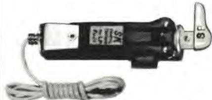
Equipped with two sapphire needles (1 and 3 mil). One needle is for 33 1/3-45 RPM, the other is for 78 RPM records. Frequency response 40 to 12,000 CPS. Needle Pressure: LP, 8 gr., SP, 8 gr. Standard 1/2" mounting holes. Includes 15" length of flexible shielded phono wire which has solderless standard connections to crystal. Individually packaged in cardboard box.
