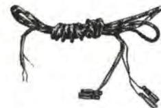
Consists of 4 color coded extremely flexible twisted wires encased in a flexible braided shield 2 foot long. Four cartridge clips attached at one end, other end stripped and tinned. Designed for use with 4 wire stereo cartridges to convert monaural tone arms for stereophonic recordings. The design of the cable insures lowest possible hum with Magnetic and Reluctance stereo cartridges. Packed individually in plastic box.
