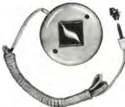
Bone conduction type magnetic receiver. Low impedance type for connection to voice coil side of output transformer, eliminating high voltage on connecting wires, as in conventional high impedance crystal type units. Automatically cuts out speaker when plugged in. Supplied complete with midget plug and two circuit jack assembly, and simple wiring instructions.
