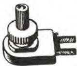
SPST rated 3 amps, 125 volts, with two 6" insulated leads.
