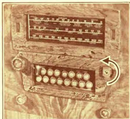
11. Then turn the set-up knob to the **LEFT** (counter clockwise). The knob will turn rather stiffly and the dial pointer will travel over to the extreme left side of the dial scale. **CONTINUE TO TURN THE SET-UP KNOB TO THE LEFT** even after the pointer reaches the end of the dial scale. **APPLY A FIRM PRESSURE UNTIL THE KNOB REACHES A DEFINITE STOP.**
