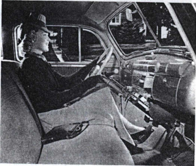
Foot switch for changing stations was a Zenith car radio tuning advance. It followed earlier innovations like the steering column tuning control.
