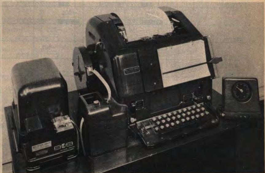
PAGE TELETYPEWRITER WITH TAPE PERFORATOR AND AUTOMATIC SENDING EQUIPMENT
