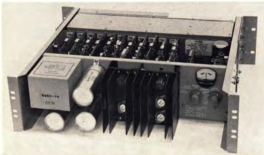
Fig. 6—The commercial unit, the AMTEC, time element compensator acts as an automatic watchman in the playback of TV tape.
