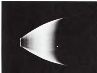
Figure 3-5. Correctly Phased Modulated R-F Envelope
