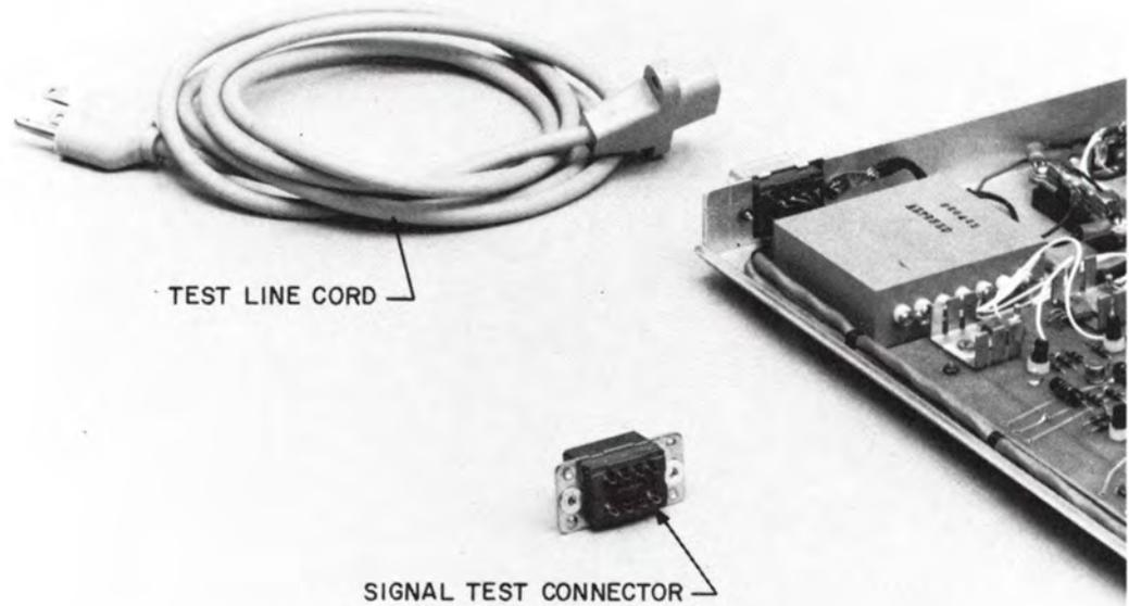
Figure 5-2. Spare Line Cord and Input/Output Connector for Test Bench Operation
