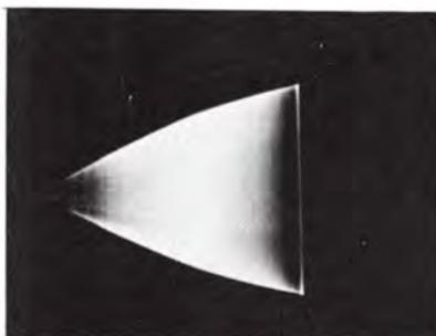
Figure 3-6. Incorrectly Phased Modulated R-F Envelope
