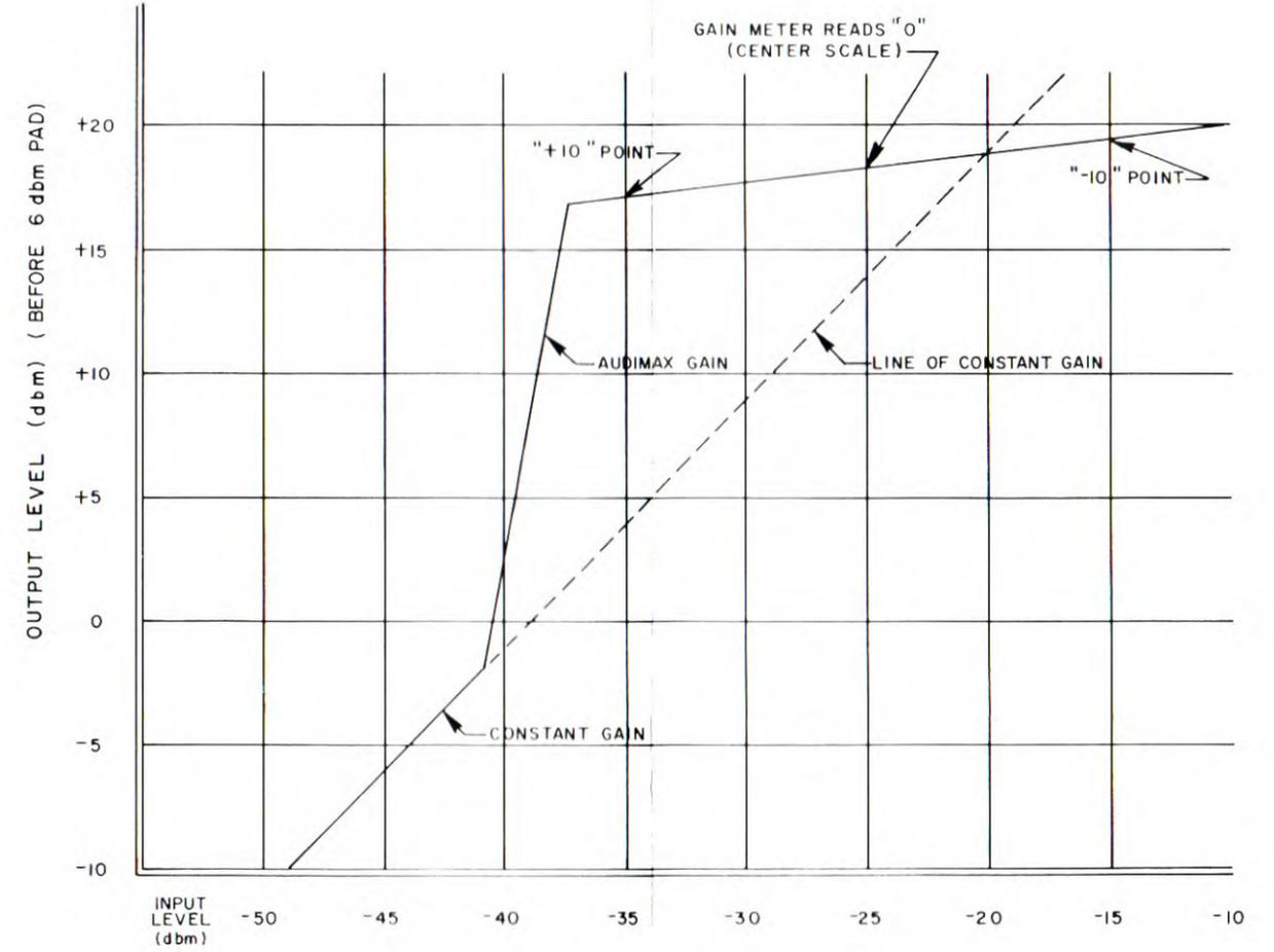
E. INPUT VS OUTPUT (dbm)
