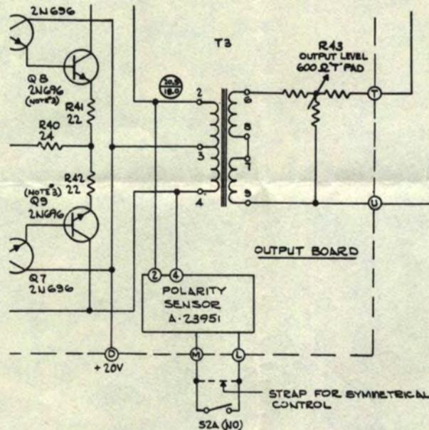
To install this new Polarity Sensor, remove the present one on the Output Board, and replace it with this new version. When soldering, make sure the points M, L, 2 and 4 are properly positioned. See drawing above; also refer to page 4-4 of your Volumax manual.
