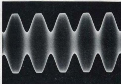
Figure 3-2. Incorrect Phasing, as Indicated by Intentionally Overdriven Volumax
