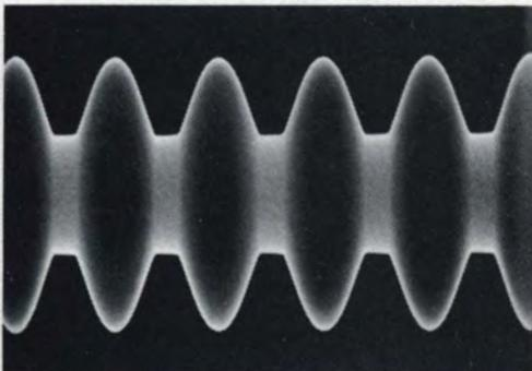
Figure 3-1. Correct Phasing, as Indicated by Intentionally Overdriven Volumax
