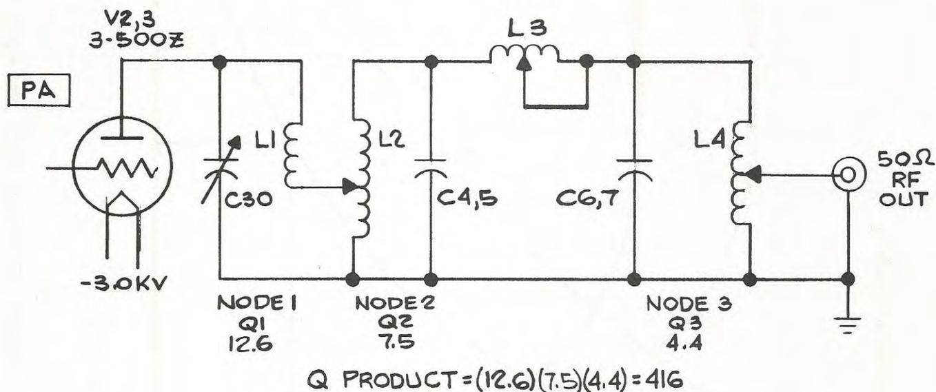
Figure 4-4. 3-Node RF Output Network.
