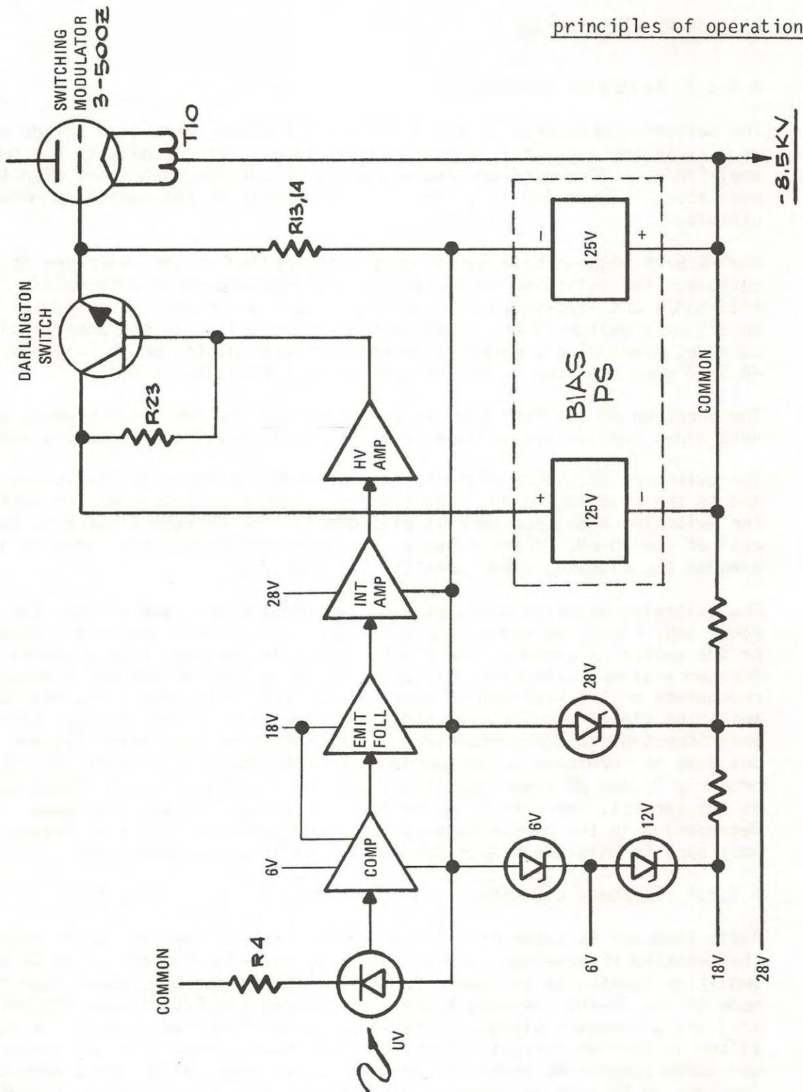
Figure 4-8. Switching Driver Operation, Block Diagram.
