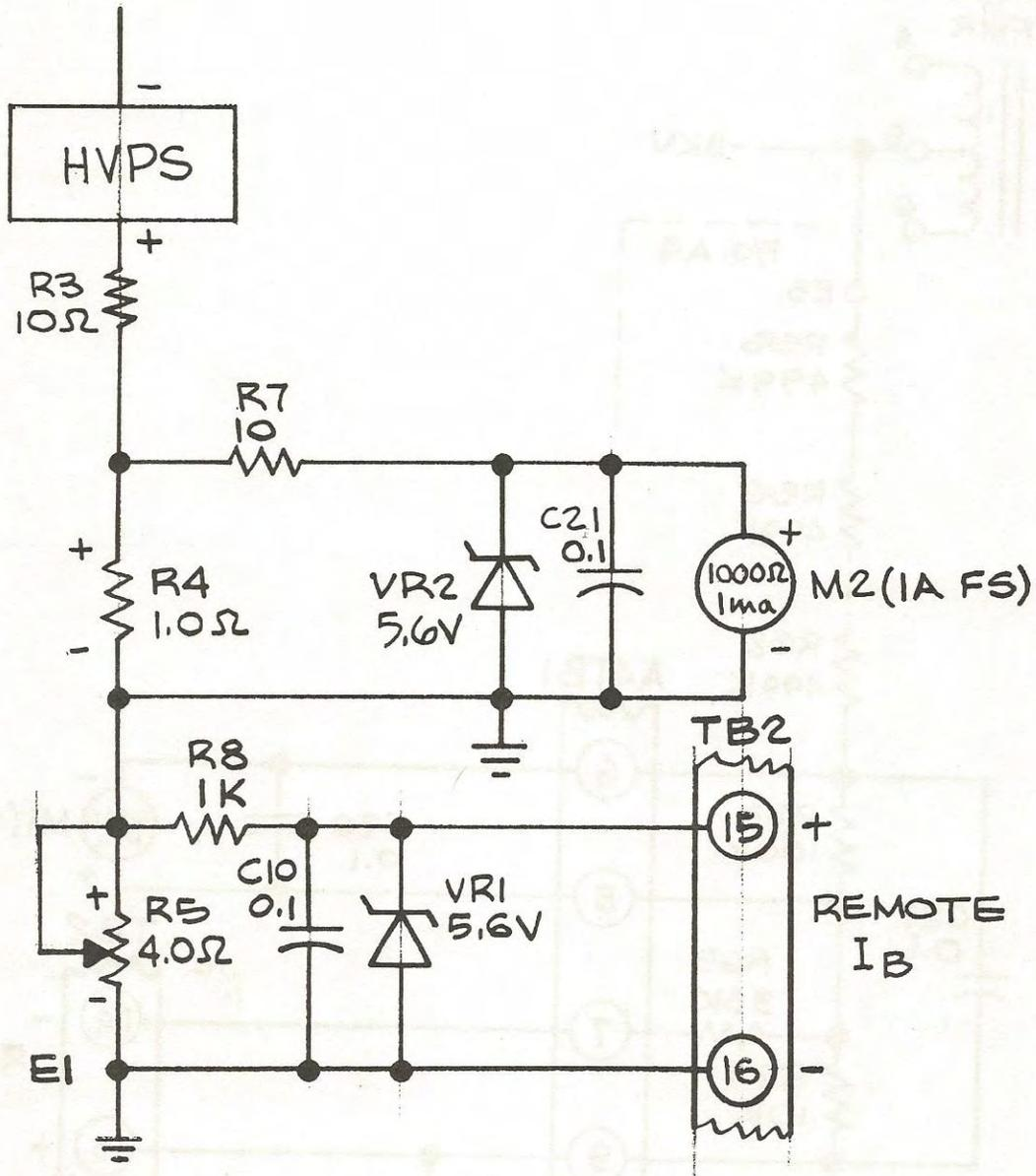
Figure 6-11. 314R-1 Plate Current Metering Circuits.
