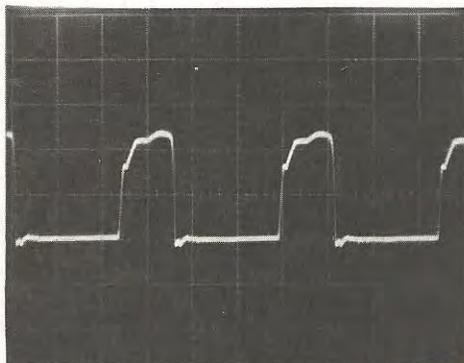
Figure 5-1. RF Exciter Output Waveform
