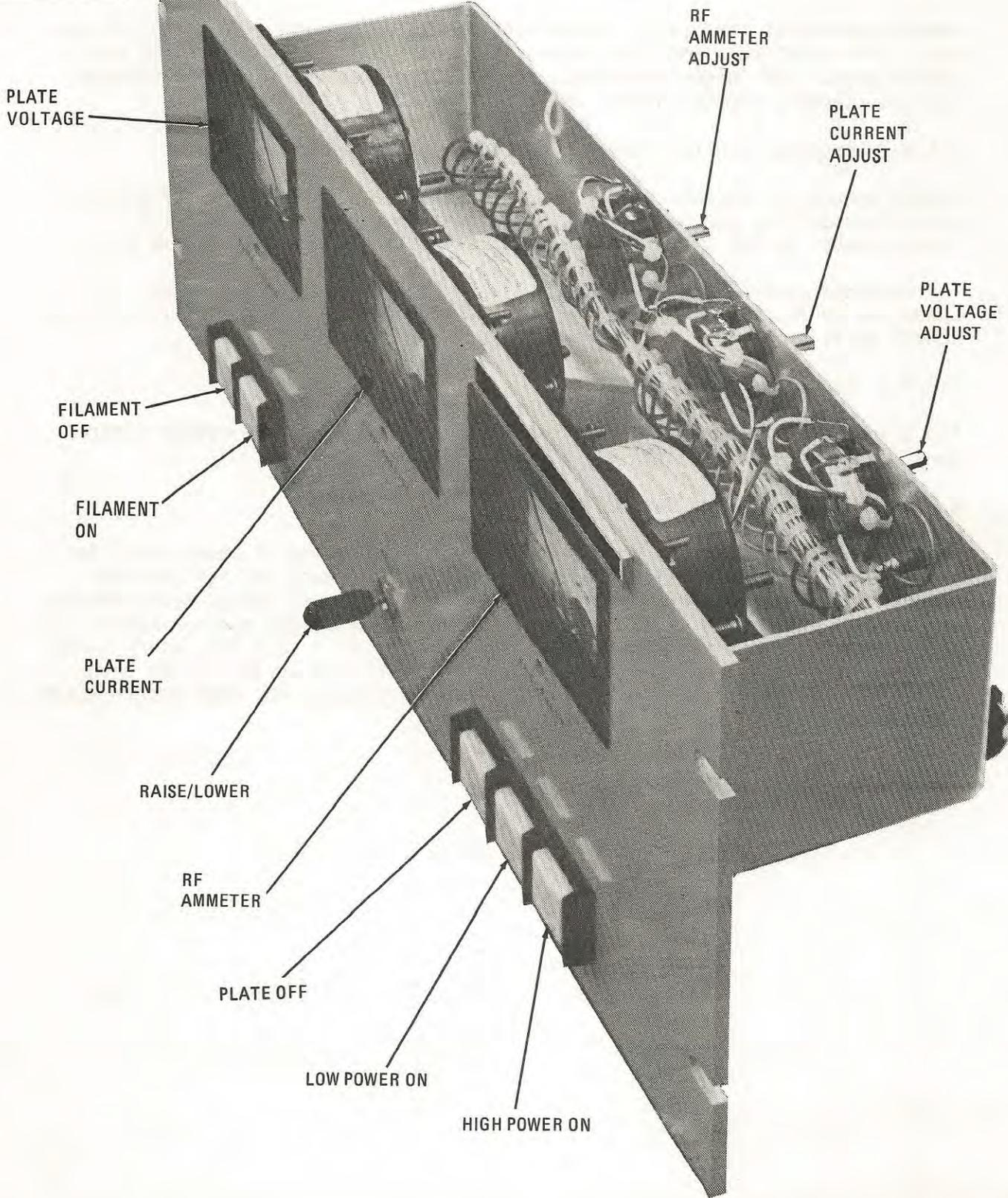
Figure 2-4. Extended Control Panel
