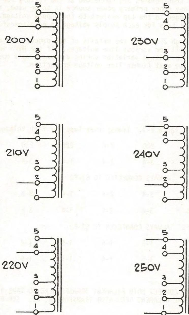
Figure 2-2. Primary Connections For T1, T4, and T5.
