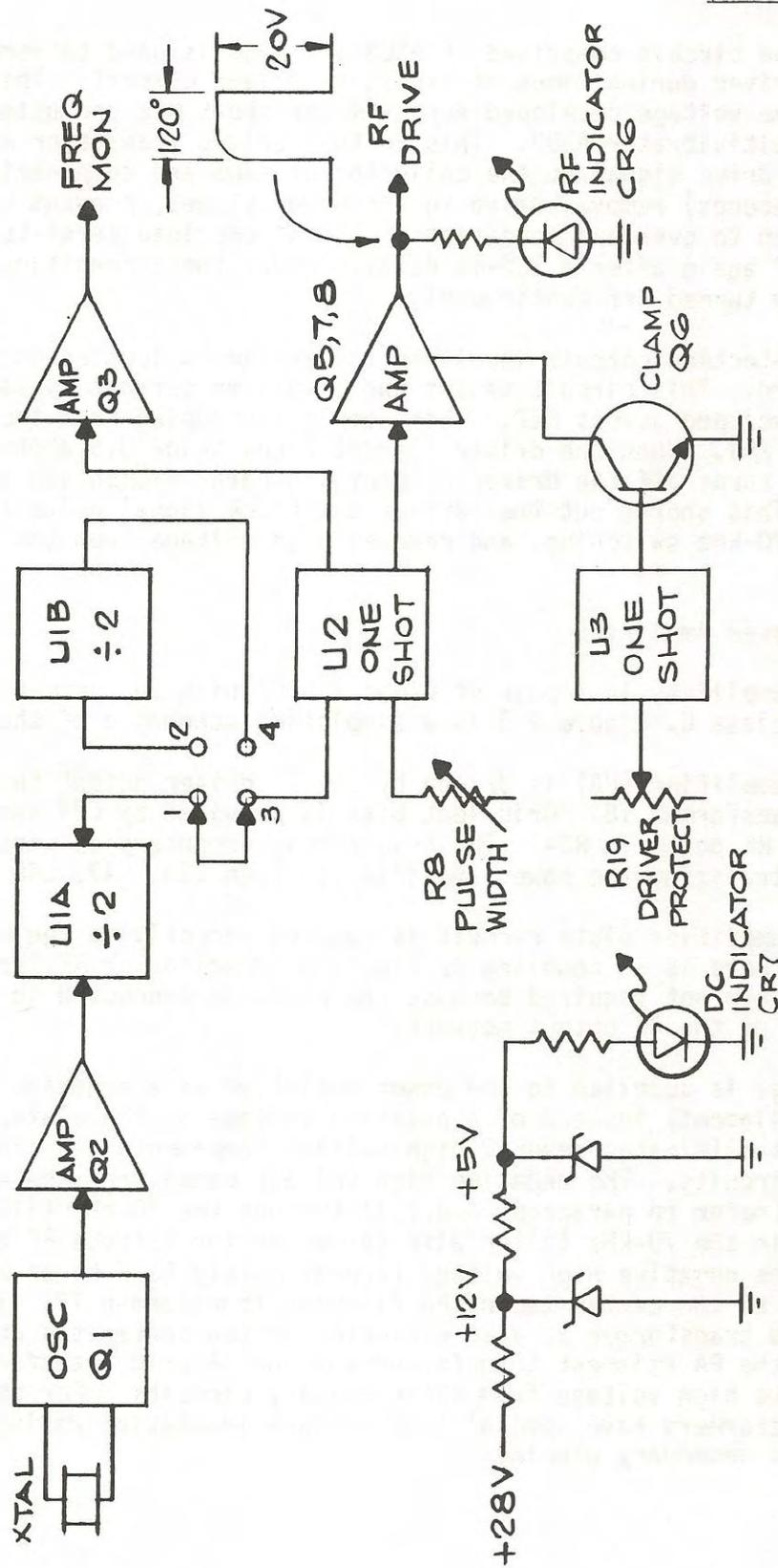
Figure 4-2. RF Exciter Block Diagram.
