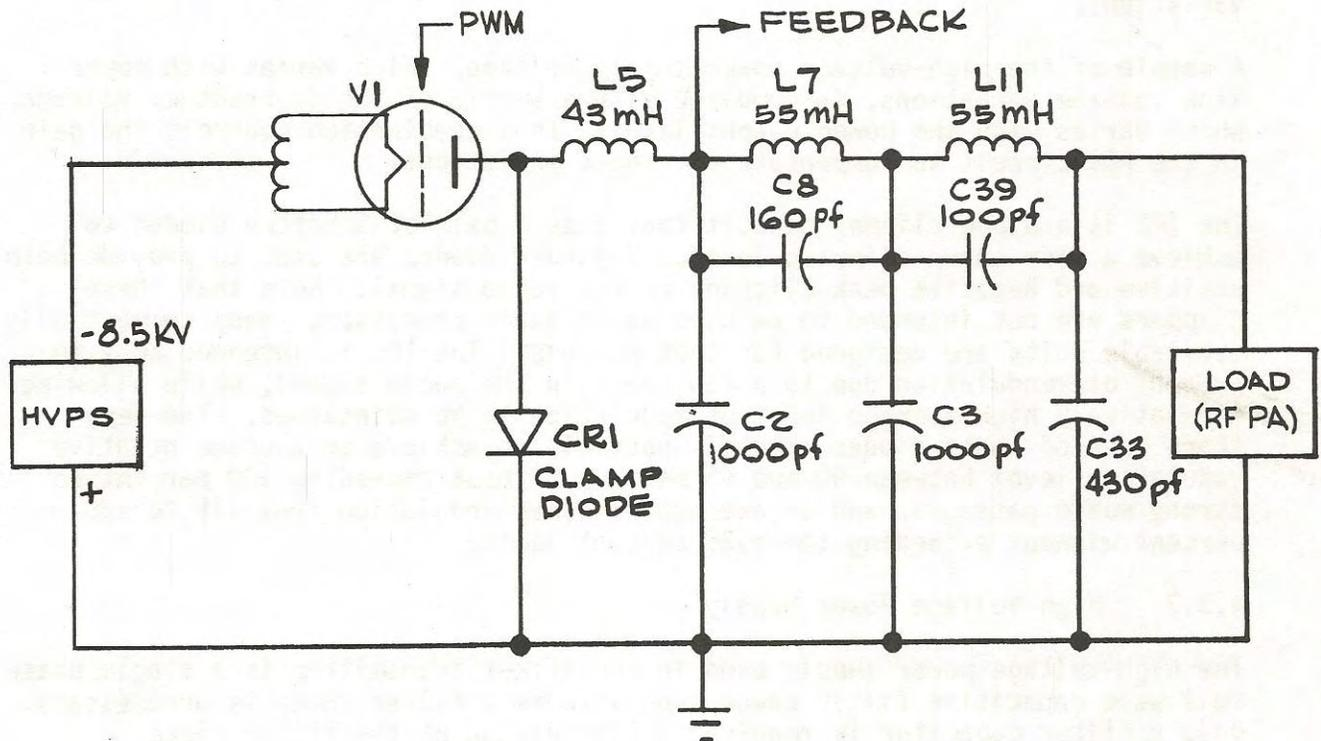
Figure 4-9. Switching Modulator Circuit.
