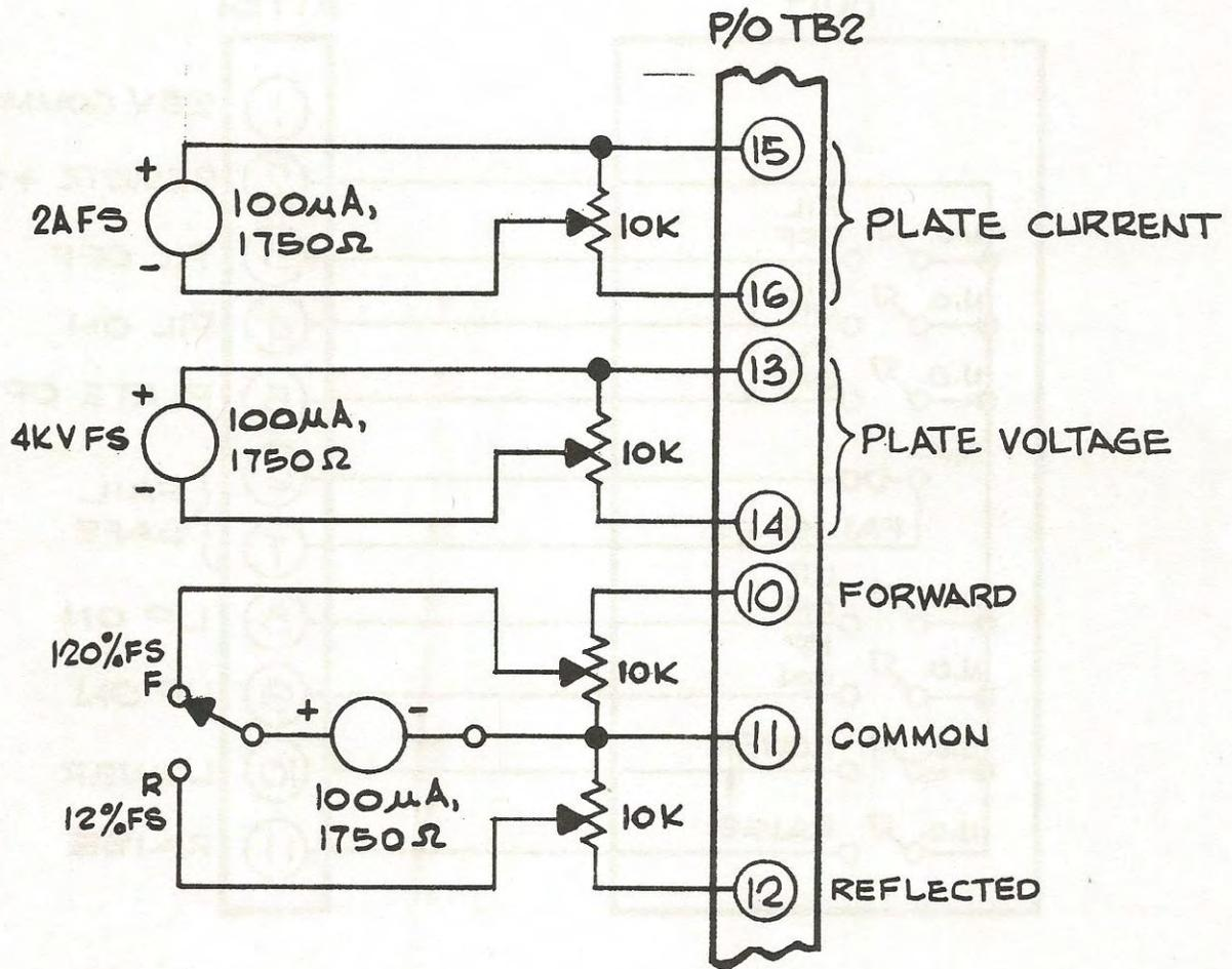
Figure 2-8. Remote Monitor Connections.
