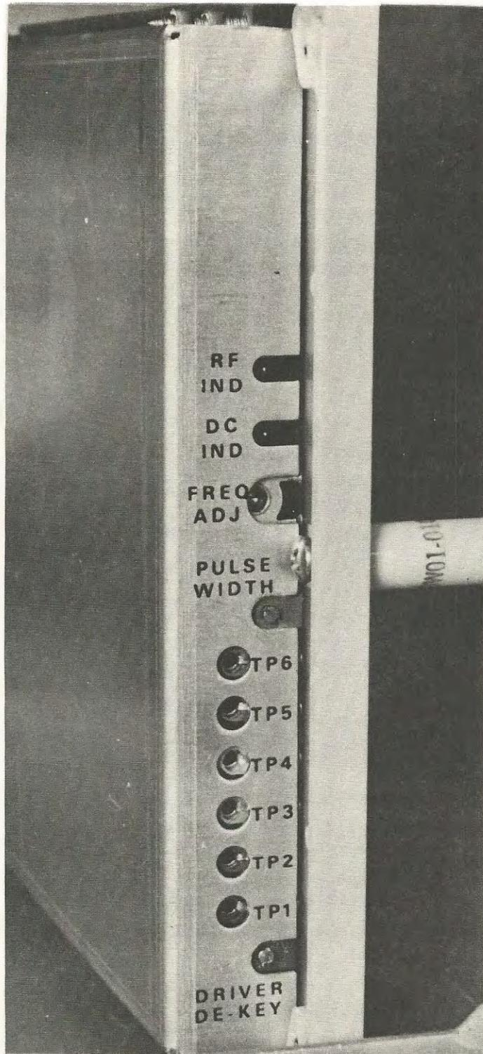
Figure 5-2. RF Exciter Front Panel
