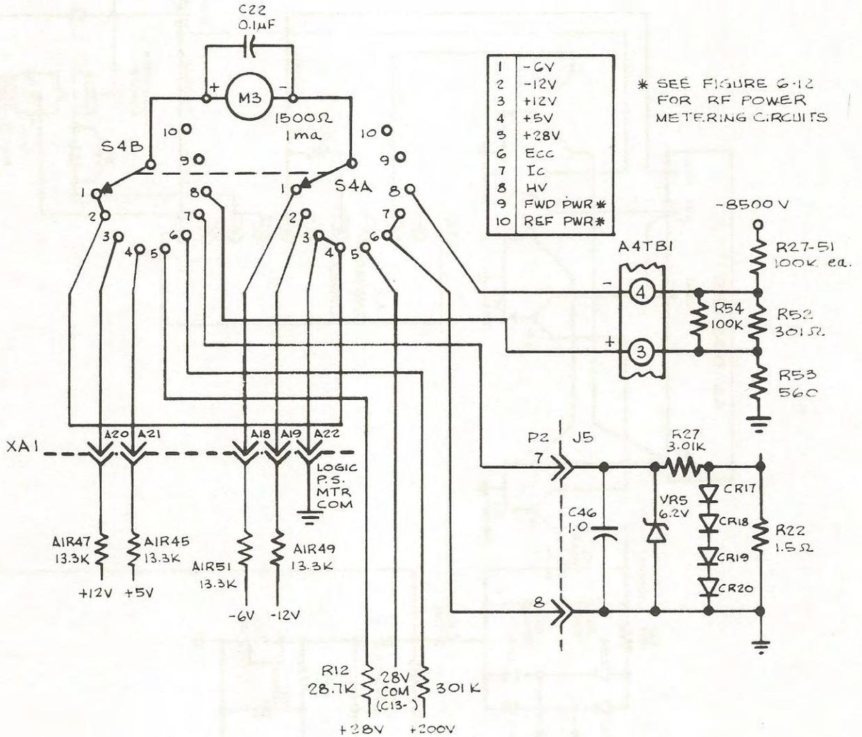
Figure 9. 314R-1 DC Metering Circuits.
