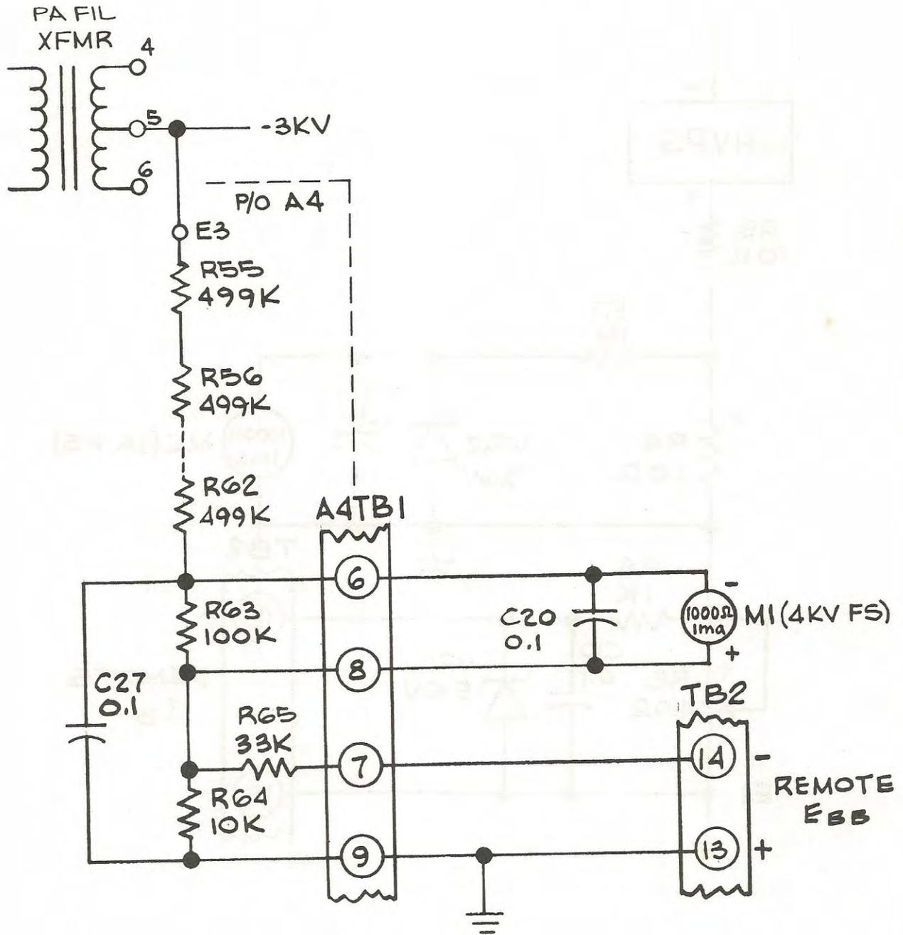
Figure 10. 314R-1 Plate Voltage Metering Circuits.
