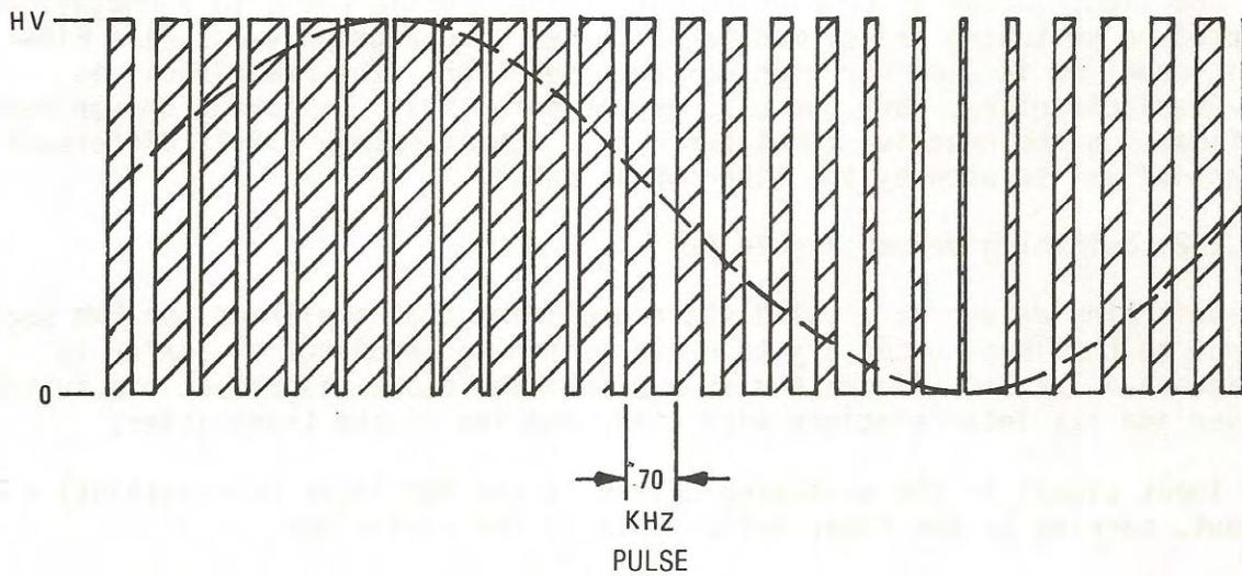
Figure 4-7. Typical PWM Waveform.
