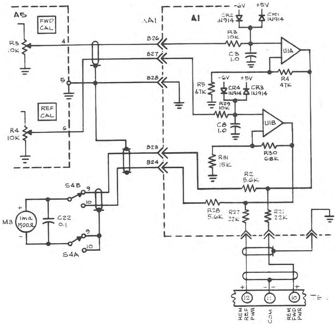
Figure 12. 314R-1 RF Power Metering Circuits.
