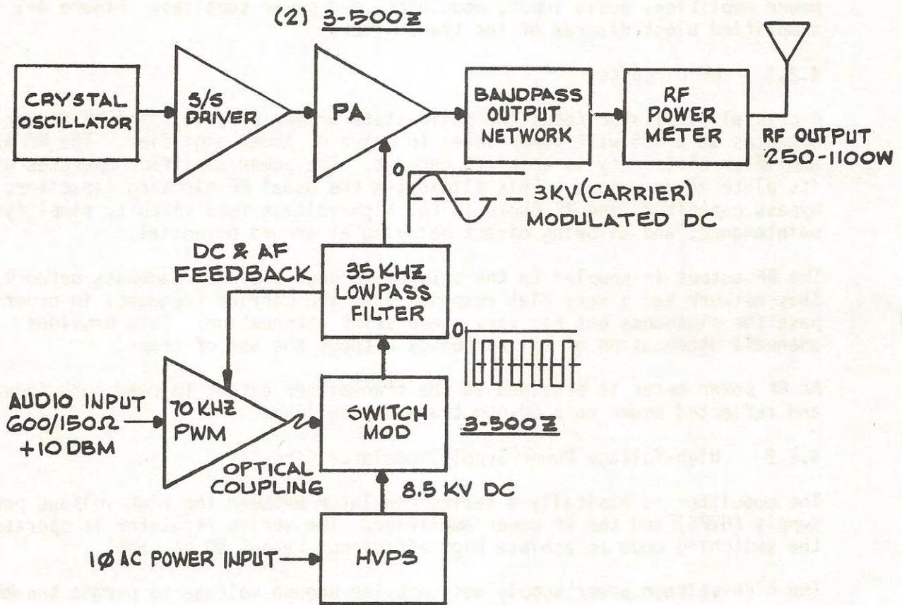
Figure 4-1. 314R-1 Simplified Block Diagram.
