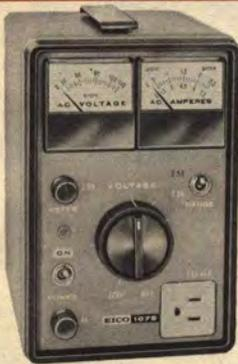
To check performance under varying line conditions—to check power consumption—to compensate for power line voltage variations—to expose intermittent components by inducing failure with over-voltage.
