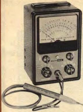
**DC VOLTMETER:** Ranges: 0.3, 15, 75, 300, 1500 volts (to 30 kv with HVP probe using 1090 megohms Multiplier Resistor). Input Impedance: 11 megohms. Accuracy:  $\pm 3\%$ .
