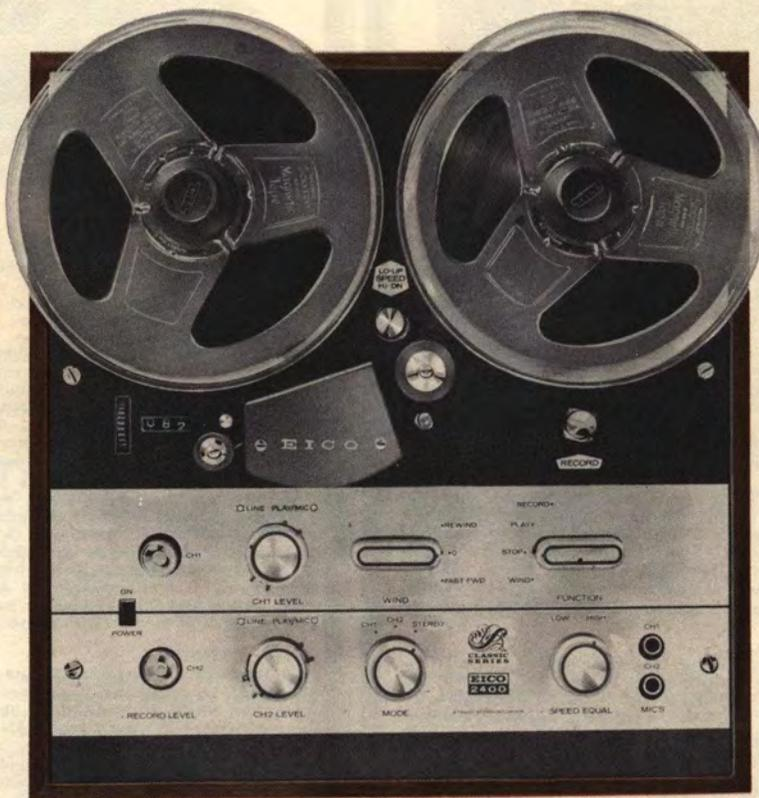
The Eico 2400 offers performance on par with tape recorders selling at more than twice the price and rivals the best in durability. Three motor design enables each motor to perform its particular function at maximum efficiency. Together, they keep tight reins on tape motion: smooth starts without tape slack, jerk or bounce—fast stops precisely controlled by DC brakes that never let tape sag or spill, never need adjustment.
