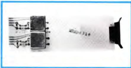
**F72537 (725 TIS) STEREO LINE LEVEL INPUT CARD**—Equivalent to two 725 TIM on a single card.
