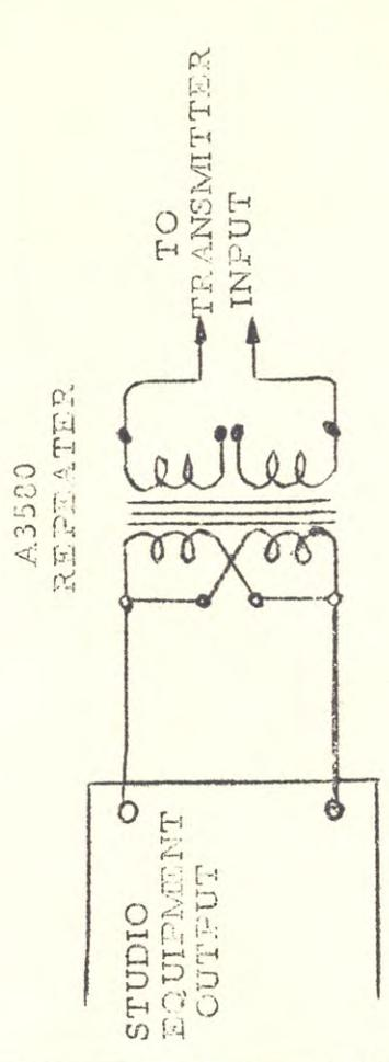
FIG. 4 - EQUALIZING THROUGH IMPEDANCE MISMATCH
