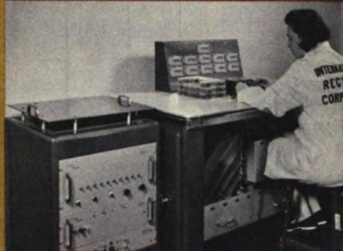
**ABOVE:** Highly sophisticated voltage reference elements for military equipment undergo electrical and physical test in lots of 100 in specially designed automated equipment shown here.
