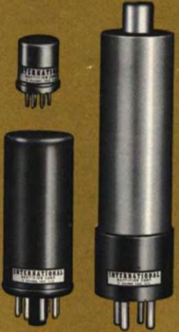
These high voltage rectifiers are specifically designed to supplant vacuum tube and mercury vapor tube rectifiers where the superior characteristics of silicon (no warm-up time, long life, high temperature operation, minimum heat generation, rugged, compact package) are desired. All devices are equipped with tube bases to allow direct replacement of their tube counterparts.
