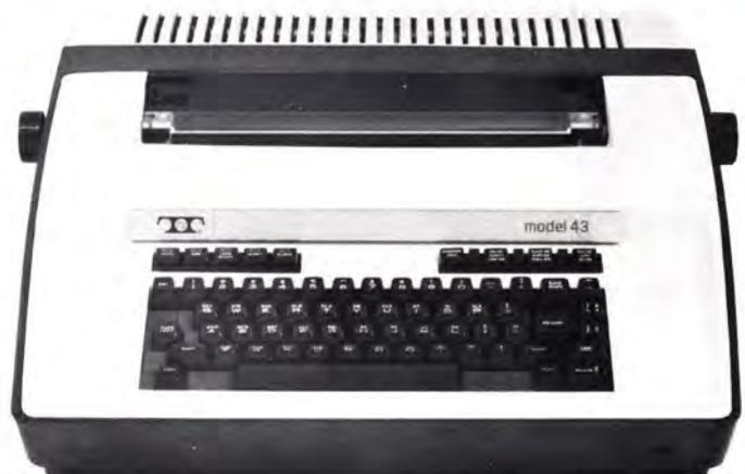
*Teletype model 43 printer with full keyboard for programming and header preparation is used in the Auto Logger option.*
