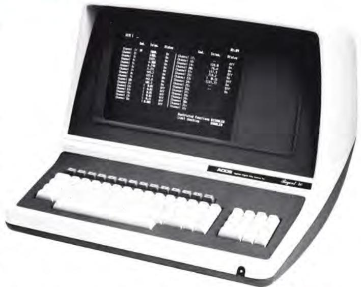
*ADDS Regent 40 terminal, used in the CRT option, duplicates full operational capabilities of the MRC-1 control terminal.*
