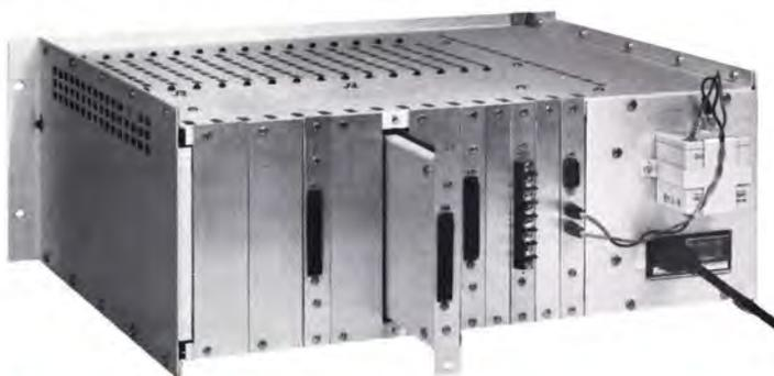
*Rear view of MRC-1 remote terminal. Plug-in interface modules are fully shielded for superior RFI suppression. A Gel Cell® battery mounted on the rear of the chassis maintains user-programmed memory during power failures.*
