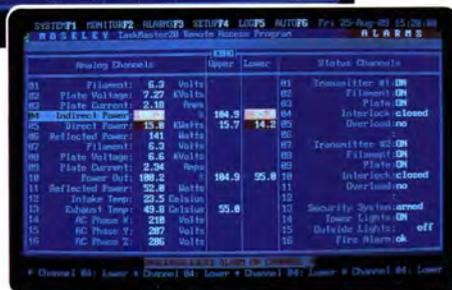
▶ Current alarm conditions are displayed and acknowledged on the Alarm Page. Up to 20 of the latest alarms and hourly log data from the last 30 hours can be logged at your convenience.
