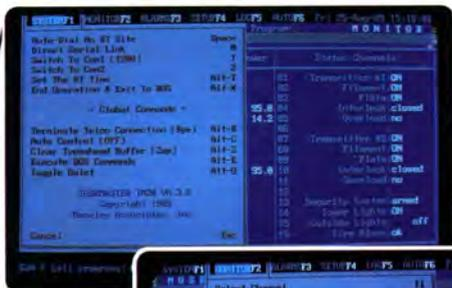
▶ The TaskMaster20 software is an easy to use software package that allows you to access and control your Remote Terminal via a PC and modem. Pull down menus are available on each screen to assist you with operation of the TaskMaster20.
