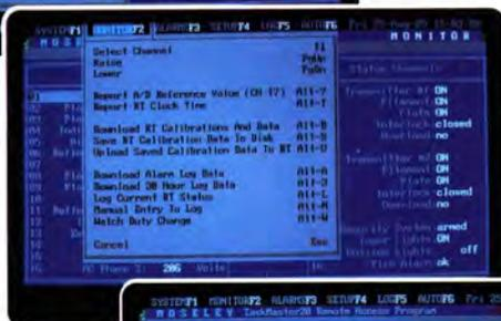
▶ The system automatically boots to the Monitor Screen for the site I.D. that you choose. The Monitor Screen allows you to view the parameters for all 16 status and telemetry channels. Use this screen to issue raise and lower commands.
