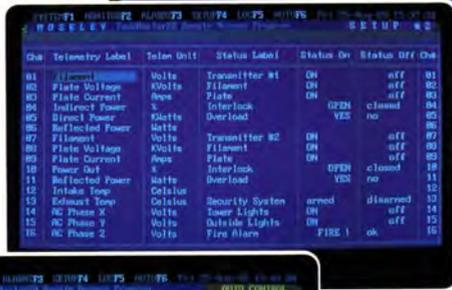
▶ You customize your own channel and status labels on the second Set-up Screen. Remote setup attributes may be uploaded or downloaded from the MRC 1620. Once you have entered your site labels, status labels and password information, you can access any site by simply entering the site I.D. with the proper password.
