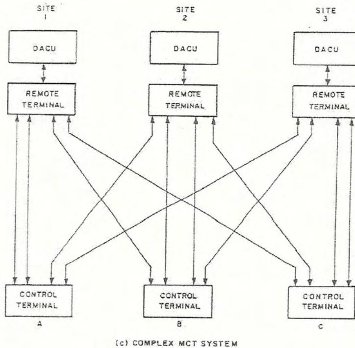
In the simple MCT system, each Control Terminal communicates independently with each Remote terminal through two data links. In the more complex MCT system, each Control Terminal talks to one Remote Terminal through two links and the other Remote terminals through a single link.
