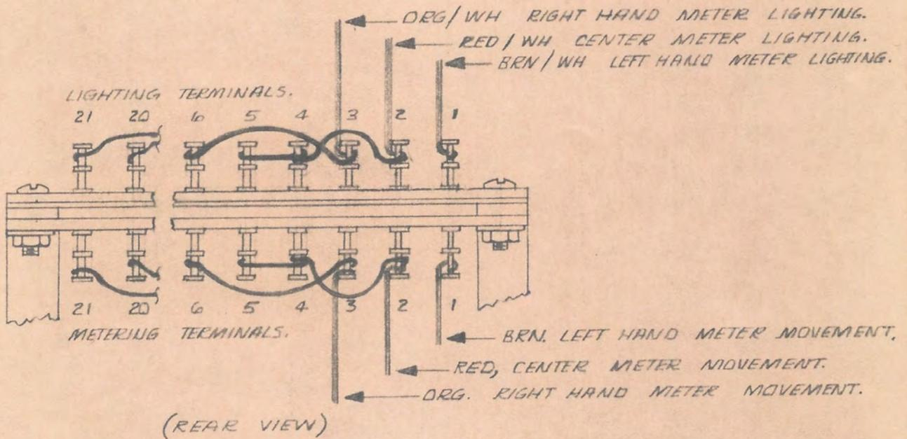
IN THIS EXAMPLE OF METER AND PUSHBUTTON ASSEMBLY WIRING, THE LEFT HAND METER (AS VIEWED FROM THE FRONT) DISPLAYS ONLY READINGS TAKEN ON PUSHBUTTON NUMBER 1. THE CENTER METER DISPLAYS NUMBERS 2, 4, AND 5. THE RIGHT HAND METER DISPLAYS PUSH BUTTONS 3 AND 6.
