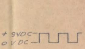
TYPICAL BINARY COLLECTOR WAVEFORM - RATE AND DUTY CYCLE WILL VARY DEPENDING ON BINARY STAGE VIEWED. CONTINUOUS CYCLING POSSIBLE BY REMOVING Q201 EACH BINARY FLIPFLOP SHOULD RUN AT 1/2 ITS OWN INPUT RATE.
