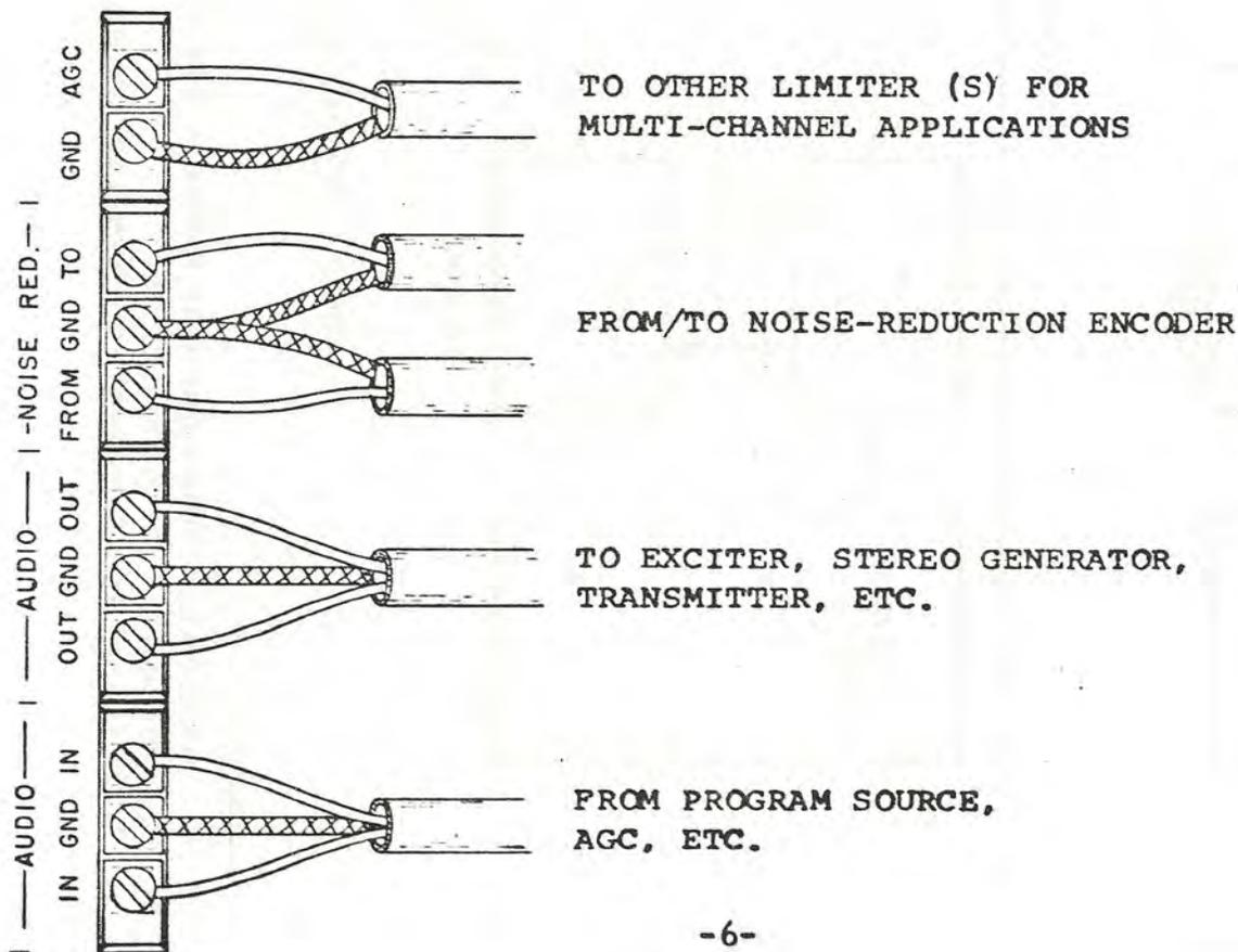
FIG. 2 - Connections to the TFL-280B. In multi-channel systems, observe program channel polarities throughout the system. As an example, follow 'red=right' and 'lower=left' or any other consistent standard throughout the plant.
