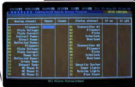
◀ Program auto-control information in the Auto Screen. Commands can be set up to be issued when a telemetry value exceeds its limits. Commands can also be initiated from a change of status condition.
