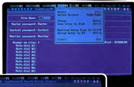
◀ A three-tiered password ("Monitor", "Control" and "Master") environment protects your system. Only the "Master" password may change set-up information. Program the Site Name and password on the first Set-up Screen. Nine (9) auto-dial numbers are also programmable to directly call out to a TaskMaster20 when alarm conditions occur.
