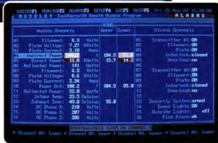
◀ Current alarm conditions are displayed and acknowledged on the Alarm Page. Up to 20 of the latest alarms and hourly log data from the last 30 hours can be logged at your convenience.
