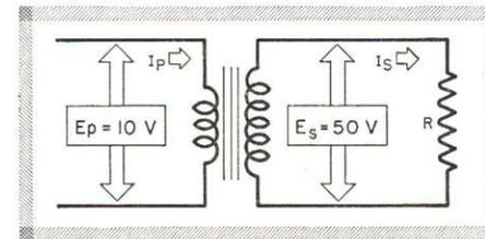
FIG. 8. A step-up transformer.
