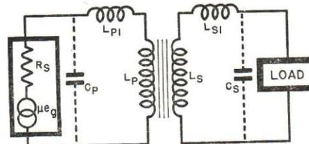
FIG. 16. The distributed capacity  $C_P$  can be made to resonate with the primary, which improves the high-frequency response up to the resonant frequency. However, above this point, there is a sharp drop in response.
