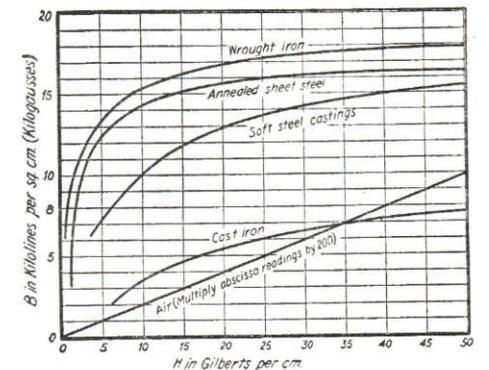
FIG. 4. B-H curves are useful to engineers because they show how various materials differ in their characteristics.
