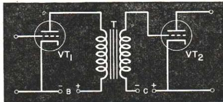
FIG. 9. Typical connections for an interstage transformer.
