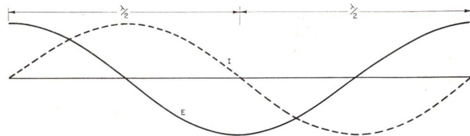
FIG. 5. Current and voltage standing waves along a full-wave wire.
