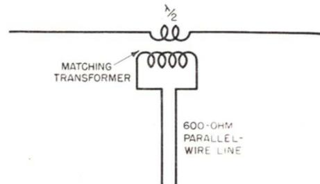
FIG. 15. A 600-ohm line can be made to appear as 72 ohms to the antenna by using an impedance-matching transformer.
