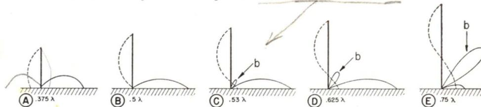
FIG. 23. Current distribution curves (dotted lines) and vertical radiation patterns (thin solid lines) at one particular frequency for grounded vertical antennas having various physical lengths.
