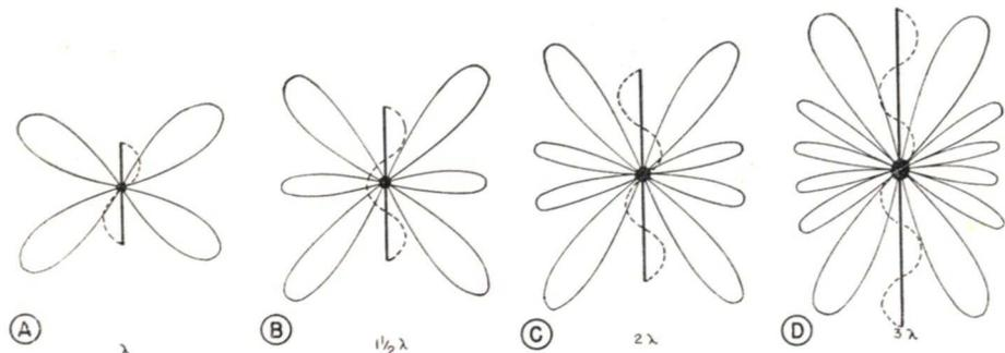
FIG. 18. Polar radiation patterns in the vertical plane (thin solid lines), and current distribution curves (thin dotted lines) for vertical antennas of various lengths in free space are shown here. You will observe that increasing the antenna length causes more of the energy to be radiated toward (but never along) the directions in which the antenna is pointing.
