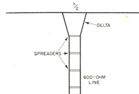
FIG. 16. The delta feed matches the line to the antenna by spreading the feeders and attaching them at the 600-ohm impedance points of the antenna.
