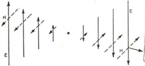
FIG. 10. An imaginary electromagnetic plane wave moving from left to right in which the electric and magnetic field lines are at right angles to each other and to the direction of wave travel.
