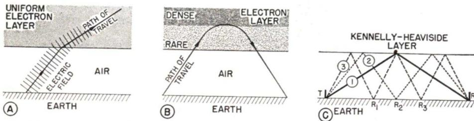
FIG. 33. These diagrams show how sky waves can be refracted (bent) back toward the earth by the Kennelly-Heaviside layer in the upper atmosphere.
