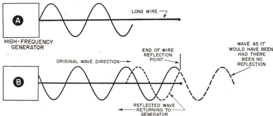
FIG. 2. Illustrating how electric waves on a wire can be reflected by the wire end. This also occurs when there is any sudden change in the wire impedance.
