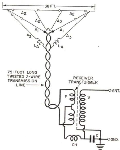
FIG. 35. All-wave noise-reducing antenna made up of three doublets. Because of its general resemblance to the web of a spider, this RCA-Victor product is commonly known as a "spider-web" antenna.
