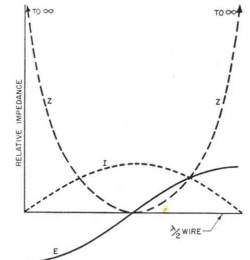
FIG. 7. The impedance at any given point along a resonant wire is equal to the voltage divided by the current at that point.
