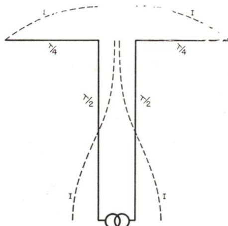
FIG. 11. Half-wave tuned feeders current-feed a remote antenna by presenting current loops at both the antenna and the transmitter.
