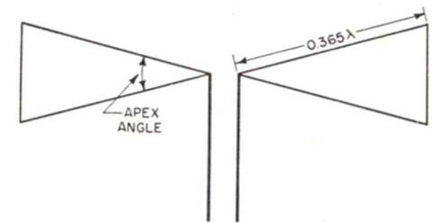
FIG. 30. The impedance of the "bi-cone" broad-band antenna can be changed by varying the apex angle of its metal cones.
