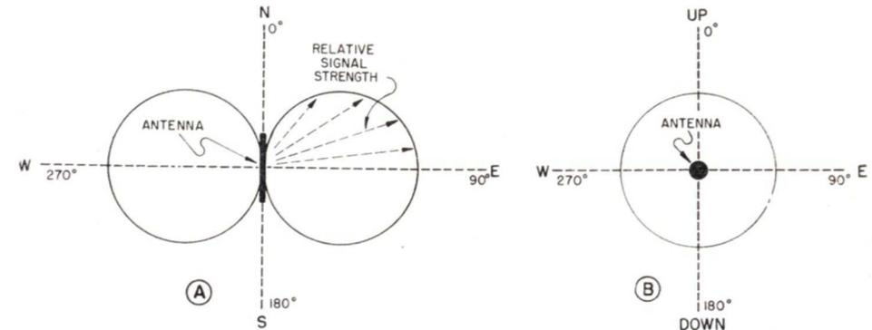
FIG. 17. In A, the horizontal plane radiation pattern for a horizontal half-wave antenna in free space resembles a figure-eight. The vertical plane pattern in B, is a perfect circle.
