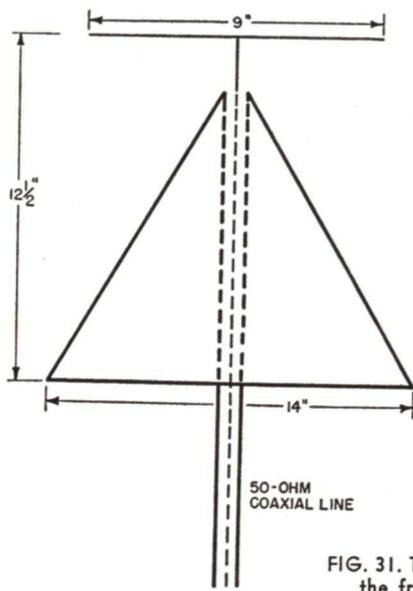
FIG. 31. This "discone" antenna matches the 50-ohm line over the frequency band 250-1000 megacycles per second.
