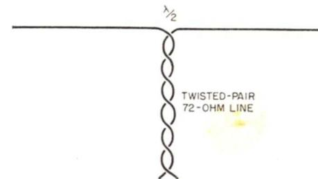
FIG. 14. A 72-ohm twisted-pair line can be connected directly to the center of a half-wave antenna without mismatch loss.
