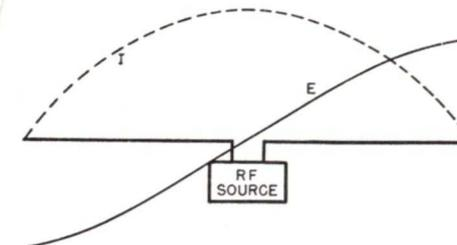
FIG. 6. Standing waves set up on a half-wave line by current-feeding at a low-impedance current loop.
