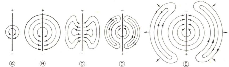
FIG. 9. The electric field is pushed into space by the next field of opposite polarity. The action of the magnetic field at right angles to the electric field (not shown) is the same.
