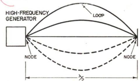
FIG. 4. Current standing waves on a half-wave wire showing the "loop" of maximum current at the center, and the zero current or "nodes" at each end.
