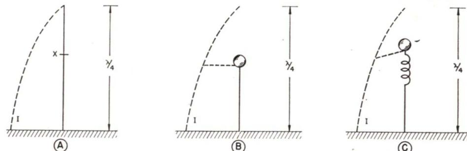
FIG. 26. Top-loading by adding capacity to the top of a short antenna can make the current distribution of the base the same as that for a true quarter-wave wire.
