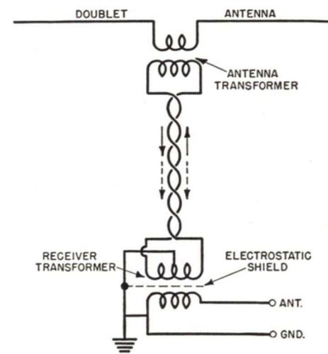
FIG. 34. A simple noise-reducing antenna.
