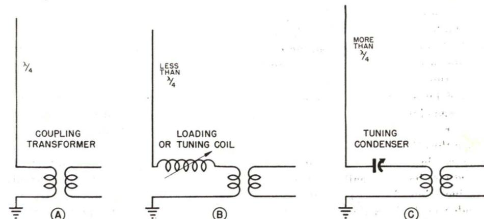
FIG. 24. Antennas that are too short or too long can be tuned to resonance by the insertion of a series-loading coil or a tuning condenser.
