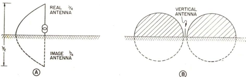
FIG. 22. A grounded vertical quarter-wave Marconi antenna together with its image appears as a complete half-wave radiator as shown in A. The vertical plane radiation pattern from such an antenna is shown in B.
