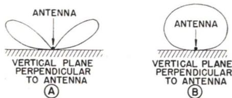
FIG. 20. How ground reflection changes the radiation pattern of a horizontal antenna.
