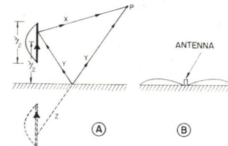
FIG. 21. An image antenna can be used with a vertical antenna to determine ground reflection effects. Note, however, that the two respective antenna currents are not reversed but are in phase. When the center of a vertical half-wave antenna is a half-wave above ground, as shown in A, it gives the vertical plane radiation pattern pictured in B.
