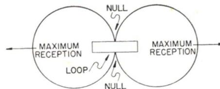
FIG. 37. Reception pattern in the horizontal plane for a vertical loop antenna. Note the extremely sharp nulls which make it useful for direction-finding.
