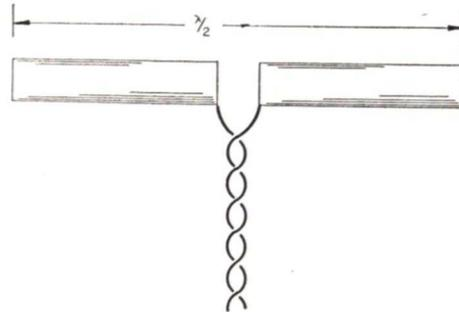
FIG. 28. Broad-banding is accomplished in the "stove-pipe" antenna by making the dipole conductors of large diameter.
