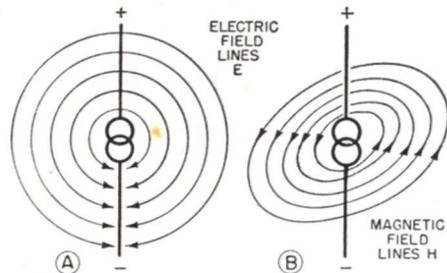
FIG. 8. The electric and magnetic field lines surrounding a resonant current-carrying conductor in free space.
