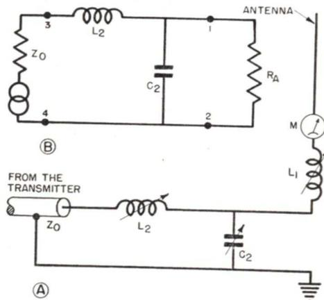
FIG. 25. In A is shown the actual circuit, and in B the equivalent circuit of a coupling network used to match a low-impedance concentric transmission line to a high-impedance antenna.
