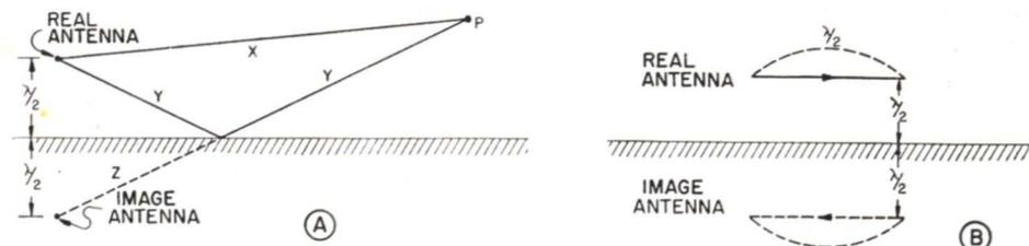
FIG. 19. How ground effects can be simulated correctly by assuming that the reflected waves are radiated by a fictitious image antenna below the ground surface.
