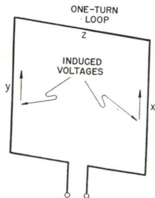
FIG. 36. A radio wave induces an e.m.f. in each side of a wire loop, and these voltages will cancel each other unless there is a difference in the time that a radio wave intercepts the two sides of the loop. For this reason, maximum signal is received when the top edge of the loop z is pointed toward the signal source.
