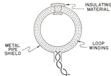
FIG. 38. A method of electrostatically shielding a loop antenna for radiomarine or aircraft use.
