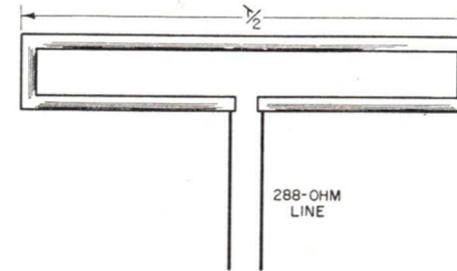
FIG. 29. The "folded dipole" is not only broad-band because of the large-diameter conductors, but it also has a built-in impedance step-up of 4 to 1 to match a high-impedance line.
