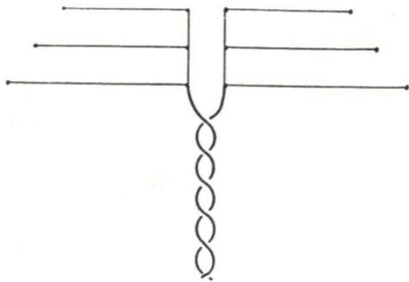
FIG. 27. Three dipoles in parallel, each of different length and resonant frequency, make up one type of broad-band antenna.
