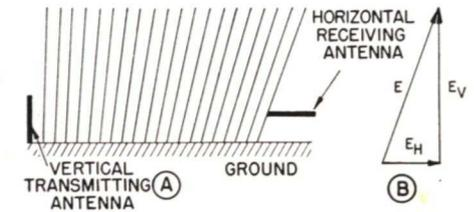
FIG. 32. Vertically polarized electric lines of force produced by a vertical transmitting antenna gradually change their angle with the ground as they travel away from the antenna.
