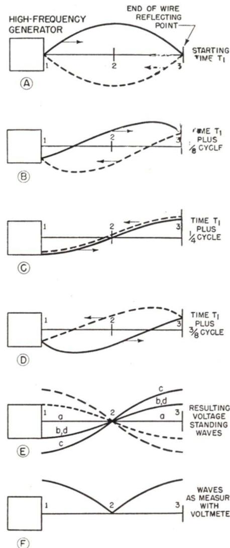
FIG. 3. Showing the manner in which original and reflected waves, traveling in opposite directions, add together to produce standing voltage waves, and how these voltage waves appear when measured with a voltmeter.
