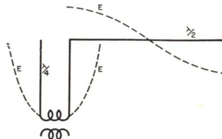
FIG. 13. The "Zepp" antenna is voltage fed.
