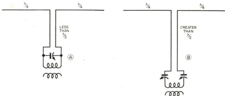
FIG. 12. For feeders that are too short, the electrical length can be increased by parallel tuning as in A. Series tuning, shown in B, is used to "shorten" feeders cut too long.
