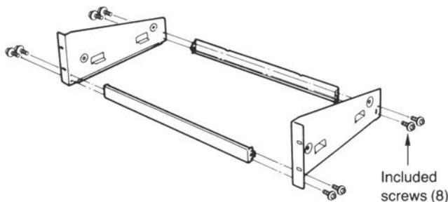
2. Remove the 4 screws on side enclosure, and attach the unit to the rack mount.
