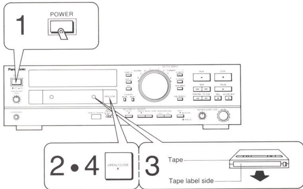
**1** Press the **POWER** Switch to switch on power.
