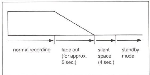
**Press the FADE OUT button during recording.**
