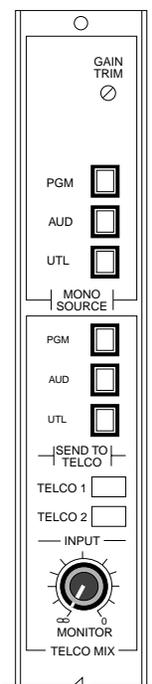
**NOTE:** The Monaural Output and Telco Mix sections of this module function independently. The Monaural Output operations are covered in Section 3.8.
