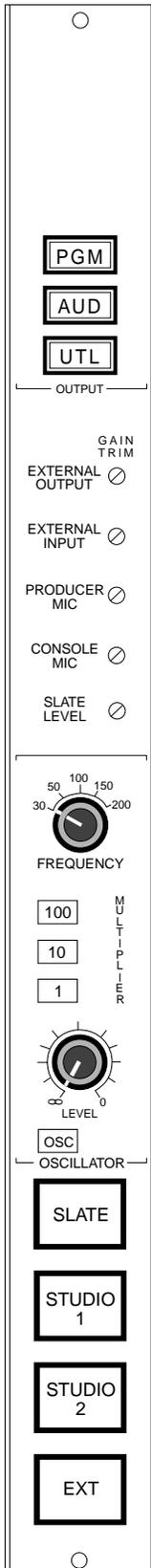
This optional module includes the independent functions for Control Room Talkback to several locations, the Producer and External Talk interfacing, a 30 Hz slate tone generator and a test tone oscillator.
