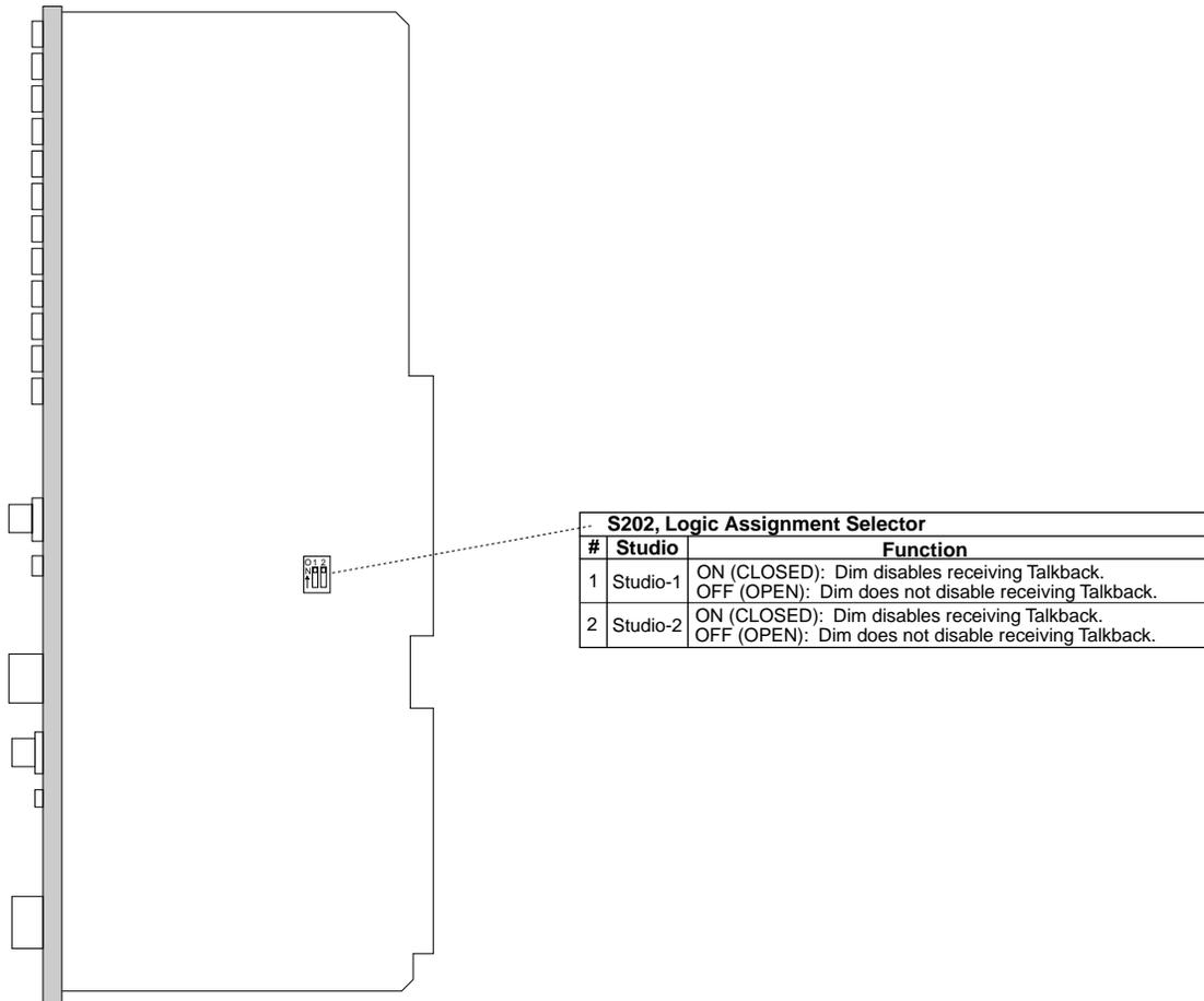
Two-station switch S202 determines how the Studio-1 and Studio-2 dim functions affect Talkback communication. Closing S202-1 causes the Studio-1 dim function to block incoming Talkback signals to Studio-1. Closing S202-2 causes the Studio-2 dim function to block incoming Talkback signals to Studio-2. Since the dim function is the result of the studio talking to another location, this function prevents other locations from talking to the studio while it is talking.
