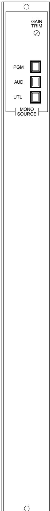
This optional module includes the Source Selection for the Mono Main and Aux Outputs and the gain trim for these outputs.
