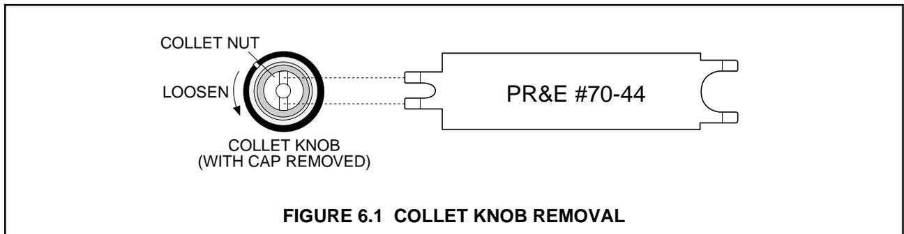
Once the nut is loosened, the collet should release from the shaft. This nut should not need to be removed unless the collet refuses to release.
