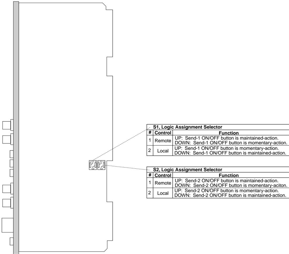
Two-station switch S1 sets whether the Send-1 local and/or remote ON/OFF buttons are momentary or maintained-action. When momentary-action is selected for the local and/or remote ON/OFF buttons, Send-1 is active only as long as the button is held depressed.
