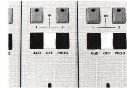
It is important to note that the operator has 2 separate means of initiating the CUE mode. One in the normal fashion of potting down and one via the push button switch located directly below the linear fader. He may go directly to cue without having to change the mixer setting.
