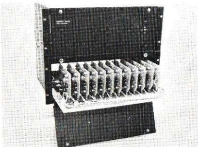
The control head has been designed for the same lightning fast access. Push two buttons and the front lip swings down. Next swing the rear hood back and you have complete access to all components and the plug in mixer mods.
