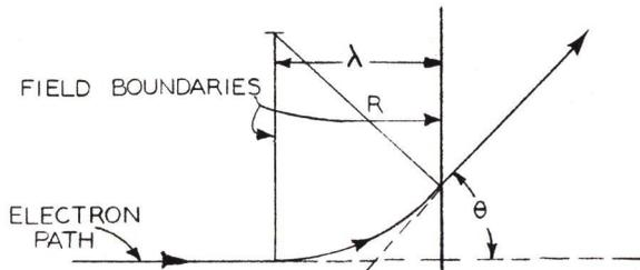
Figure 3-40 - Electron Path at Field Boundary
