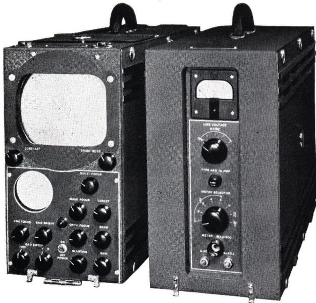
Field Camera Control and Field Power Supply
