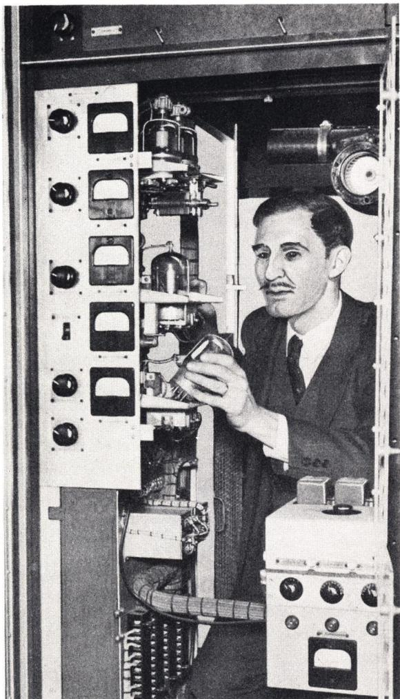
Figure 6-2 - Low-power Stages of Picture Transmitter mounted in frame 7, just below the grid-circuit of the picture PA. Note the crystal oscillator unit in box at lower right. This contains three crystals, one of which is not visible in this view. These consist of the regular video-channel crystal, a spare crystal of the same frequency, and a "tune-up" crystal of mid-band frequency.
