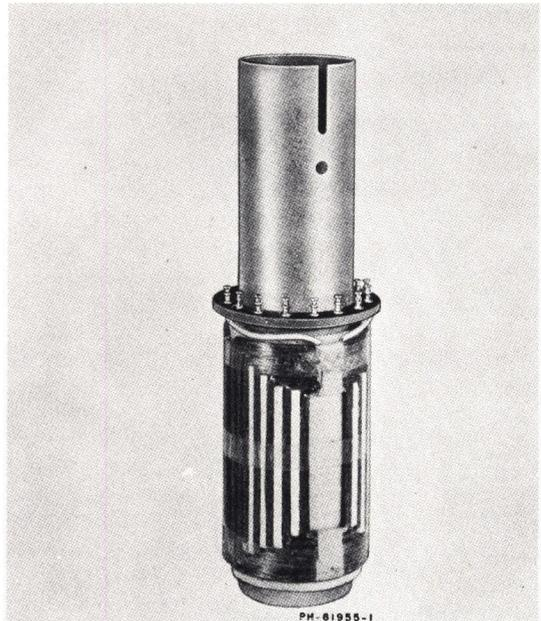
Figure 2-8 - Deflecting-coil Assembly for the Image Orthicon (Outer Tube Removed)
