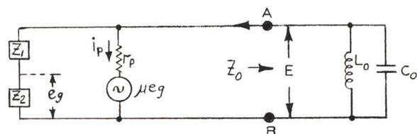
Figure 3-33 - Reactance Tube Equivalent Circuit
