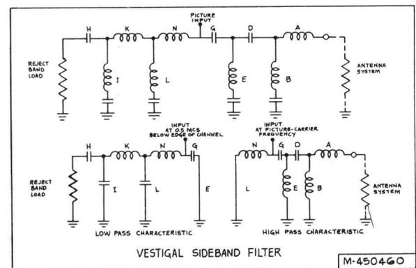
Figure 7-8 - Vestigial Sideband Filter Circuit
