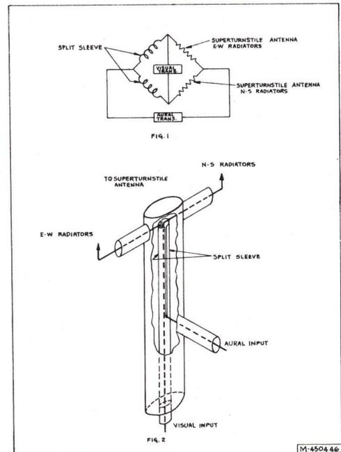
Figure 7-12 - Diplexer Schematic Diagram
