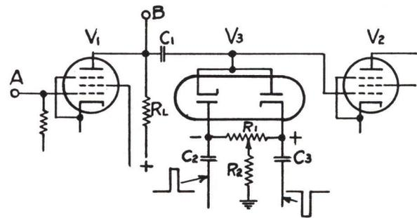
Figure 2-17 - Schematic Diagram of Clamp Circuit
