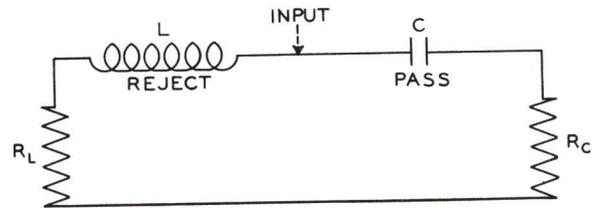
Figure 7-7 - Elementary Filter Circuit
