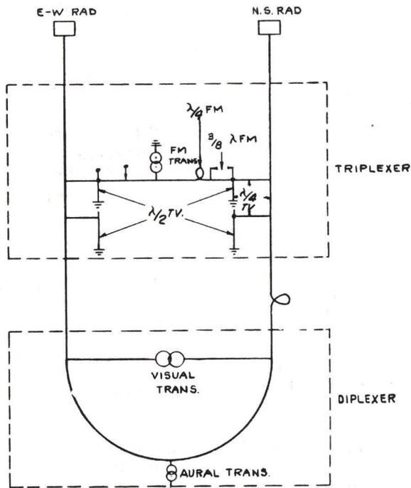
Figure 7-20 - Principle of Triplexing
