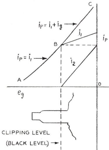
Figure 3-25 - Linear Clipper Characteristic
