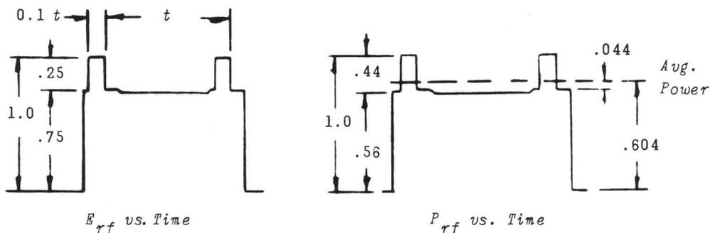
Figure 5-3 - Voltage and Power Relations for Negative Transmission
