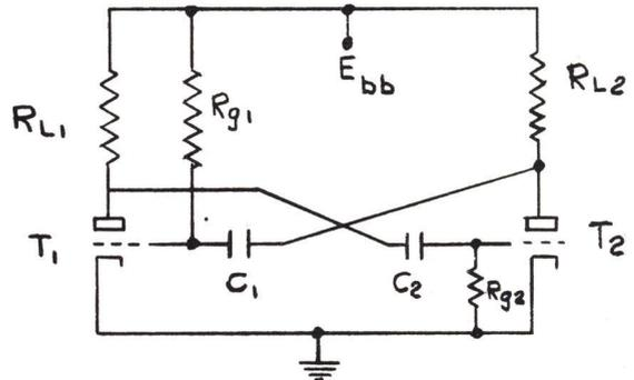
Figure 3-17 - Grid Return Circuit
