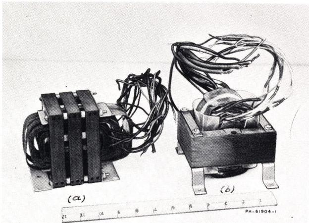
Figure 2-12 - (a) Prewar Design of a Forced-air-cooled Power Transformer. (b) New Design.
