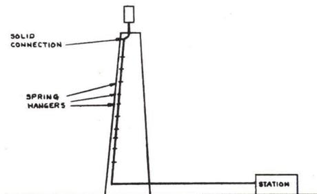
Figure 7-26 - Transmission Line Installation Layout
