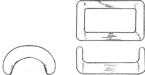
Figure 3-41 - Deflection Yoke Winding
