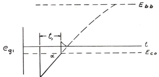
Figure 3-18 - Grid Voltage Wave Form
