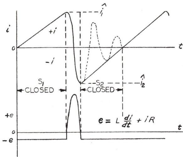
Figure 3-46 - Deflection-cycle Waveshapes
