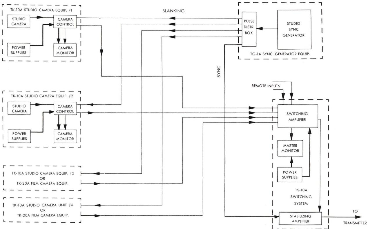
Block Diagram showing Schematic Arrangement of Studio Pickup and Control Room Equipment
