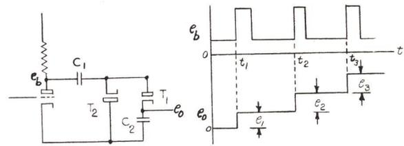
Figure 3-28 - Step-charging Circuit
