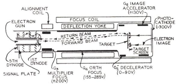
Figure 3-67 - Image Orthicon Pick-up Tube
