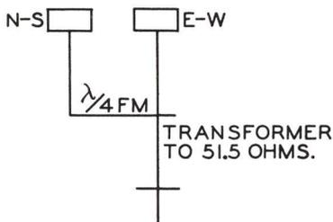
Figure 7-21 - TV Superturnstile Antenna
