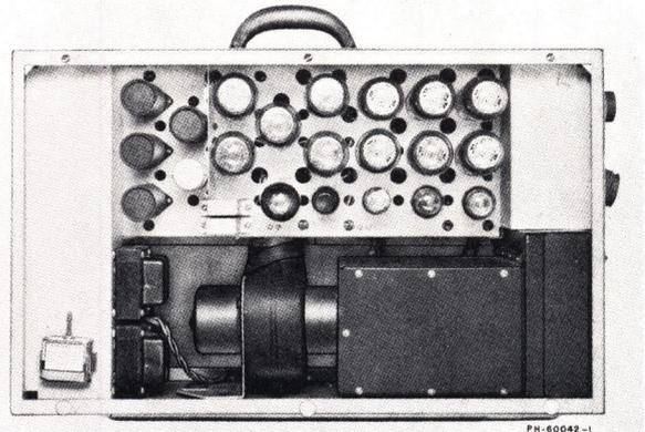
Figure 2-13 - Field Power Supply, Tube Side
