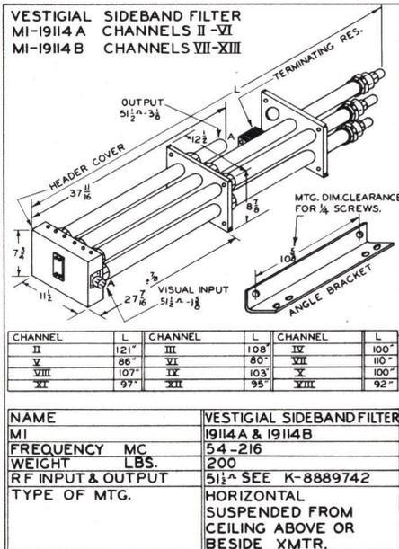
Figure 7-9 - Vestigial Sideband Filter Construction
