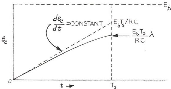
Figure 3-36 - Analysis of Sawtooth Voltage
