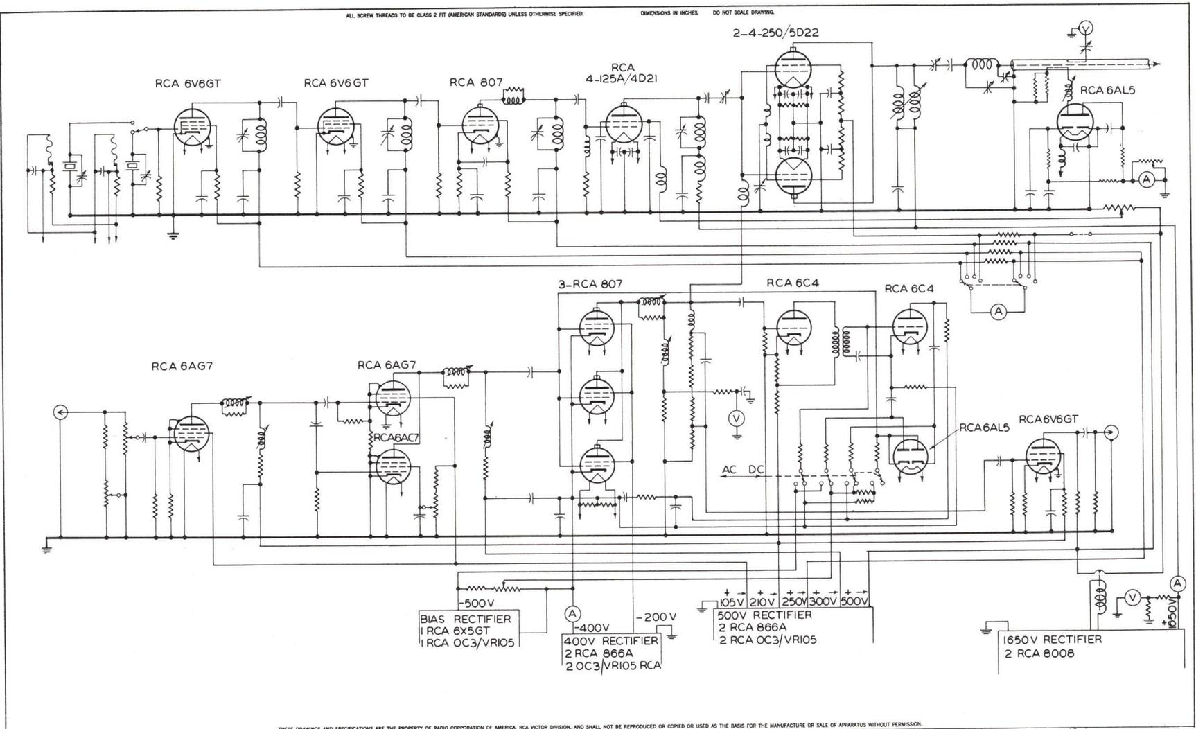
Figure 6-13 - 77-500A Transmitter, Visual Portion, Schematic Diagram (T-619060)
