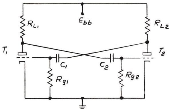
Figure 3-14 - Unbiased Free-running Multivibrator
