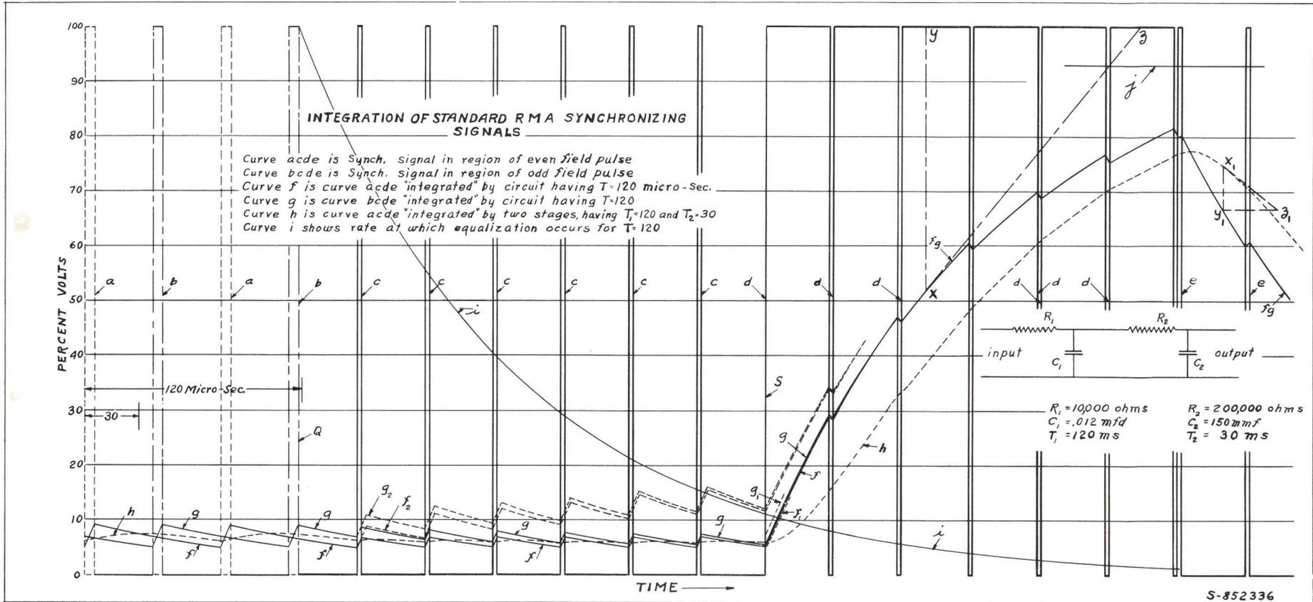
Figure 3-8 - Integration of RMA Synchronizing Signals
