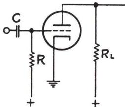
Figure 2-19 - Schematic Diagram of Differentiating Circuit
