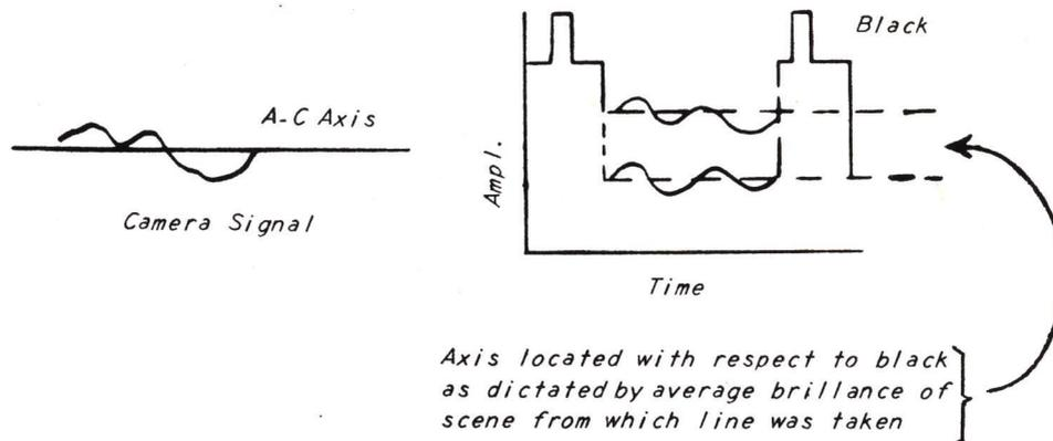
Figure 5-4 - Picture Signal Showing D-C Component
