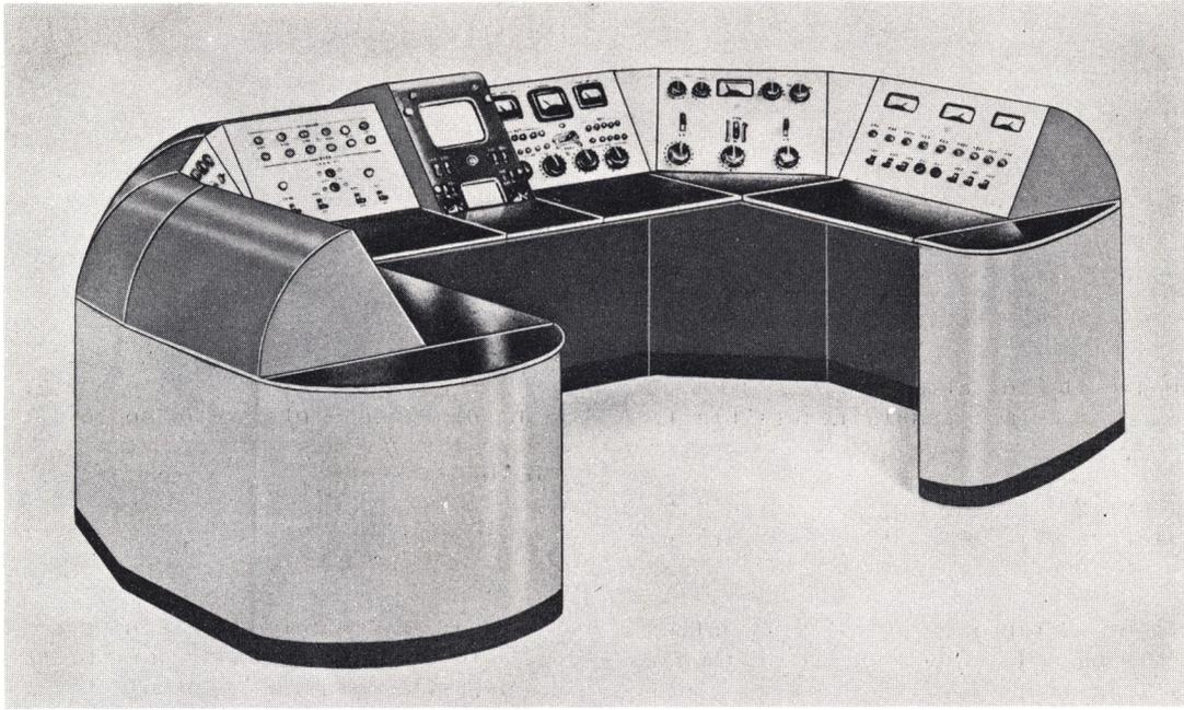
Figure 6-6 - Combination Consoles may be set up for control of any number of different types of transmitters. The above console set-up will handle a TV, an FM, and an AM transmitter.
