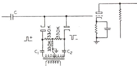
Figure 3-60 - Clamp Circuit
