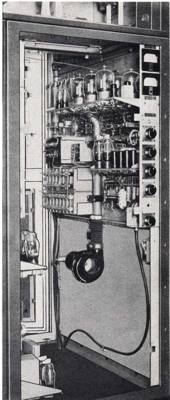
*Figure 6-4 - Video Modulator Unit. Compact and Relatively simple, this unit includes three straightforward video stages (the last of which develops all the video power needed fully to modulate the RCA-8D21 tube in the picture PA), plus the sync separator and expander circuits required in all video transmitters. By this simple, fool-proof unit, high-level modulation can be used, eliminating the chain of Class B linear stages which are necessary in "low-level" transmitters.*
