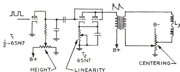
Figure 3-42 - Vertical Deflection Circuit
