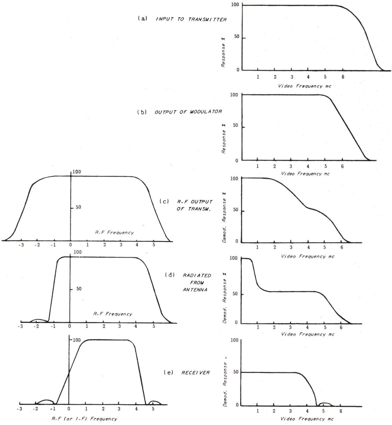
Figure 5-2 - Frequency Response Through a Television Transmitter System
