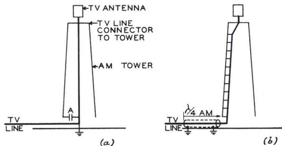
Figure 7-22 - Use of AM Tower for TV Antenna
