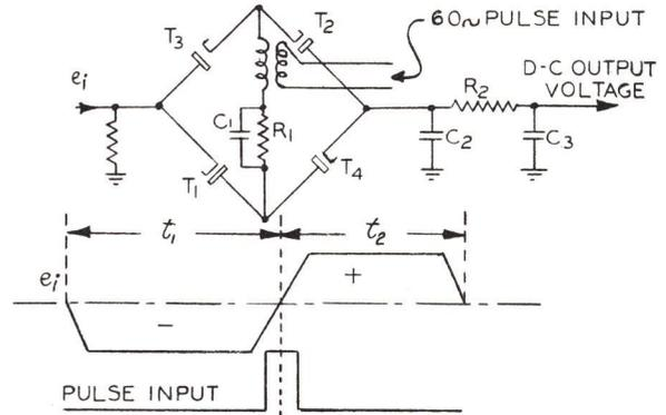
Figure 3-31 - Frequency Control Circuit
