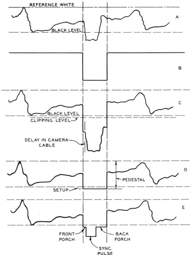
Figure 3-4 - Steps in Synthesis of Picture Signal.
