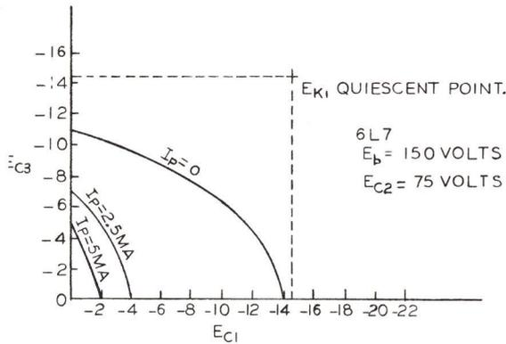
Figure 3-30 - Characteristics of Type 6L7 Tube
