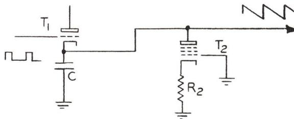
Figure 3-33 - Sawtooth Linearity Circuit
