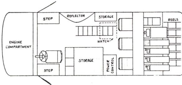
Figure 2-5 - Plan Diagram of the Mobile Unit
