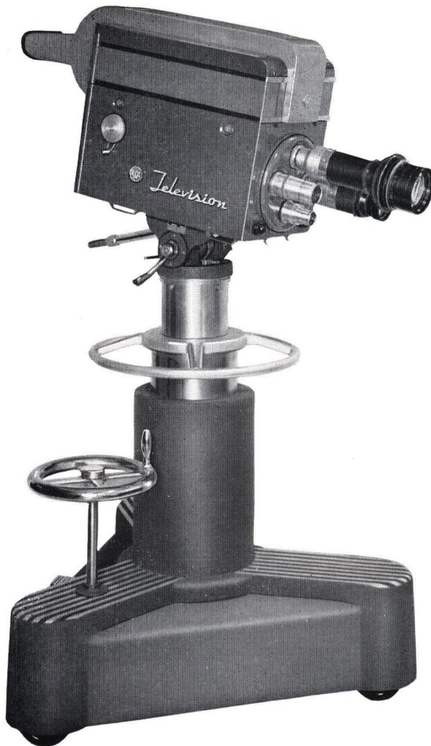
minal board below the shelf. The deflection and high voltage pulse supply circuits are mounted in a similar manner on the other side of the camera. Hinged doors on either side of the camera swing down to provide easy access to the camera circuits.
