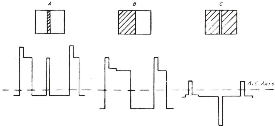
Figure 5-5 - Limiting Wave Forms in Video Signal
