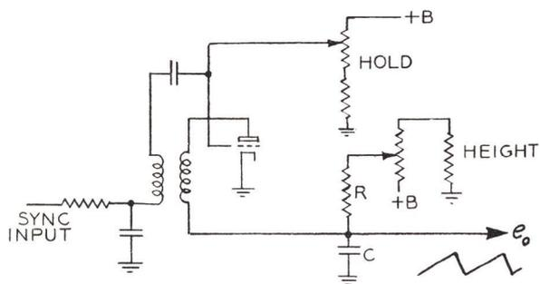
Figure 3-37 - Blocking Oscillator Sawtooth Generator
