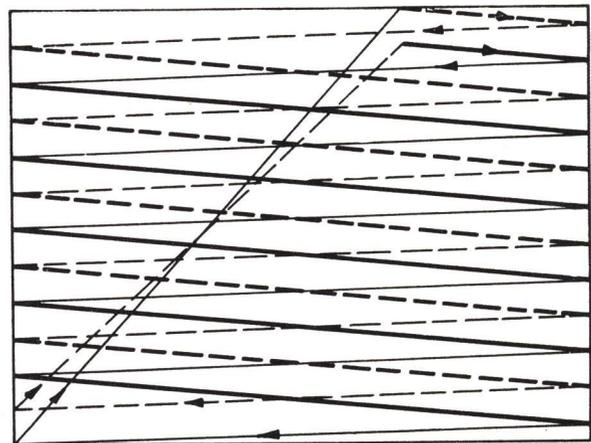
Figure 3-2 - Even line Interlaced Scanning System with 12 lines.
