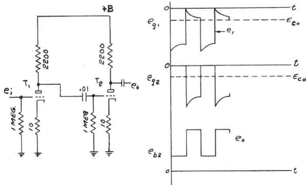
Figure 3-22 - Triode Clipper Circuit
