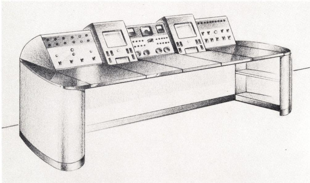
Figure 6-5 - TT-5A Television Transmitter Console
