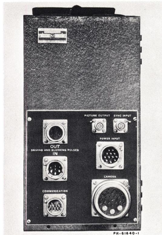
Figure 2-11 - Rear of the Camera Control
