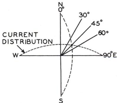
Figure 7-16 - Turnstiling Principle (Field Magnitude is Proportional to the Angle Between Direction of Radiator and Direction of Observation)
