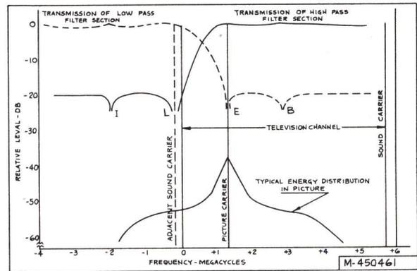
Figure 7-6 - Characteristics of Vestigial Sideband Filter
