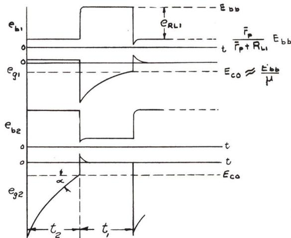
Figure 3-15 - Operating Cycle of Free-running Multivibrator
