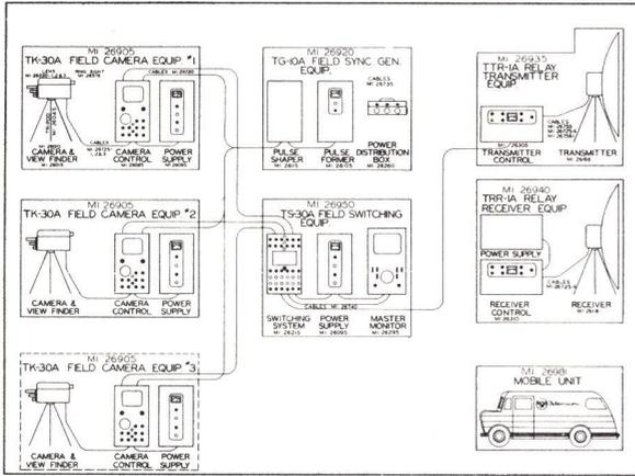
Figure 2-1 - Block Diagram of Field Pickup Equipment
