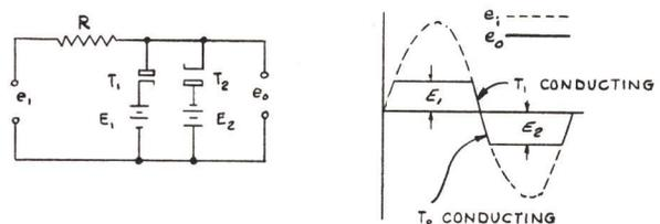
Figure 3-21 - Peak Clipping Circuit
