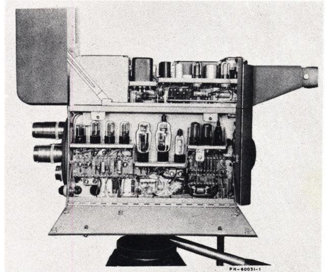
Figure 2-9 - Deflection-amplifier Side of the Camera and View Finder (Internal View)
