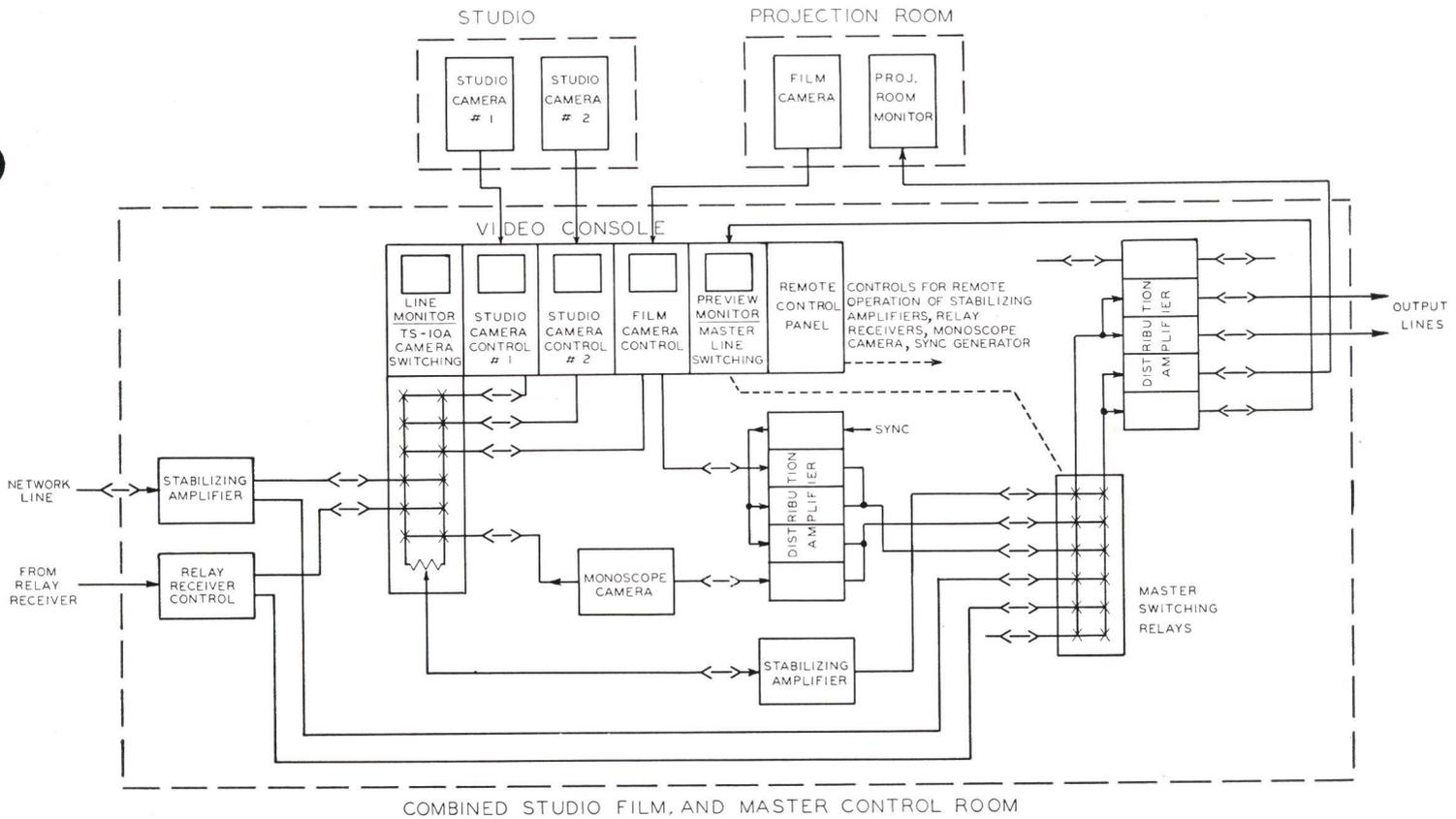
FIG. 20. Block Diagram of the Major Video Units Used in the Type C Station. Master switching in this layout is performed at the video console. Note use of video jacks for patching sources of signal into either the camera or master switching systems.
