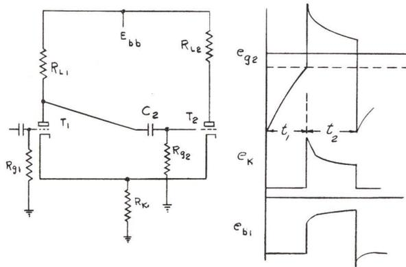
Figure 3-20 - Cathode-coupled Multivibrator
