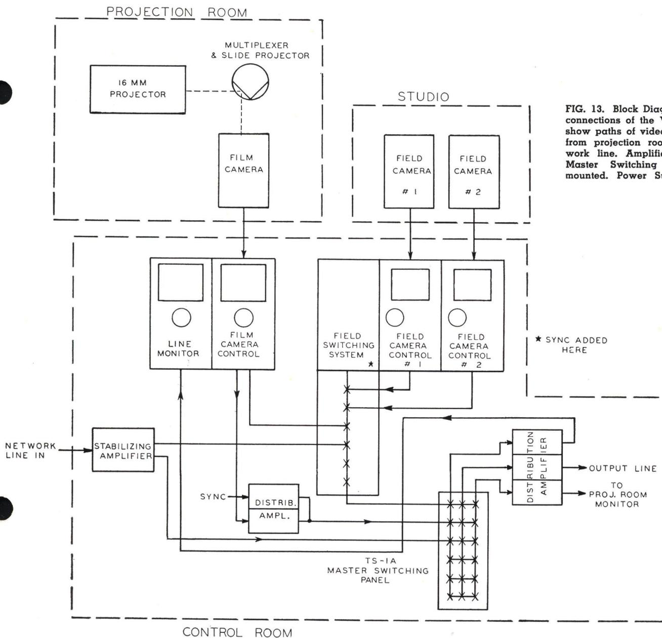
FIG. 13. Block Diagram Showing Interconnections of the Video Units. Arrows show paths of video signals emanating from projection room, studio and network line. Amplifiers and the TS-1A Master Switching Panel are rack-mounted. Power Supplies not shown.
