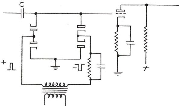
Figure 3-62 - Clamp Circuit for Single-polarity Keying Pulses
