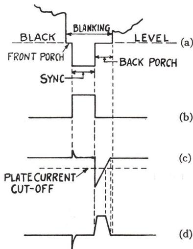
Figure 2-18 - Derivation of Keying Pulses for Back-porch Clamping
