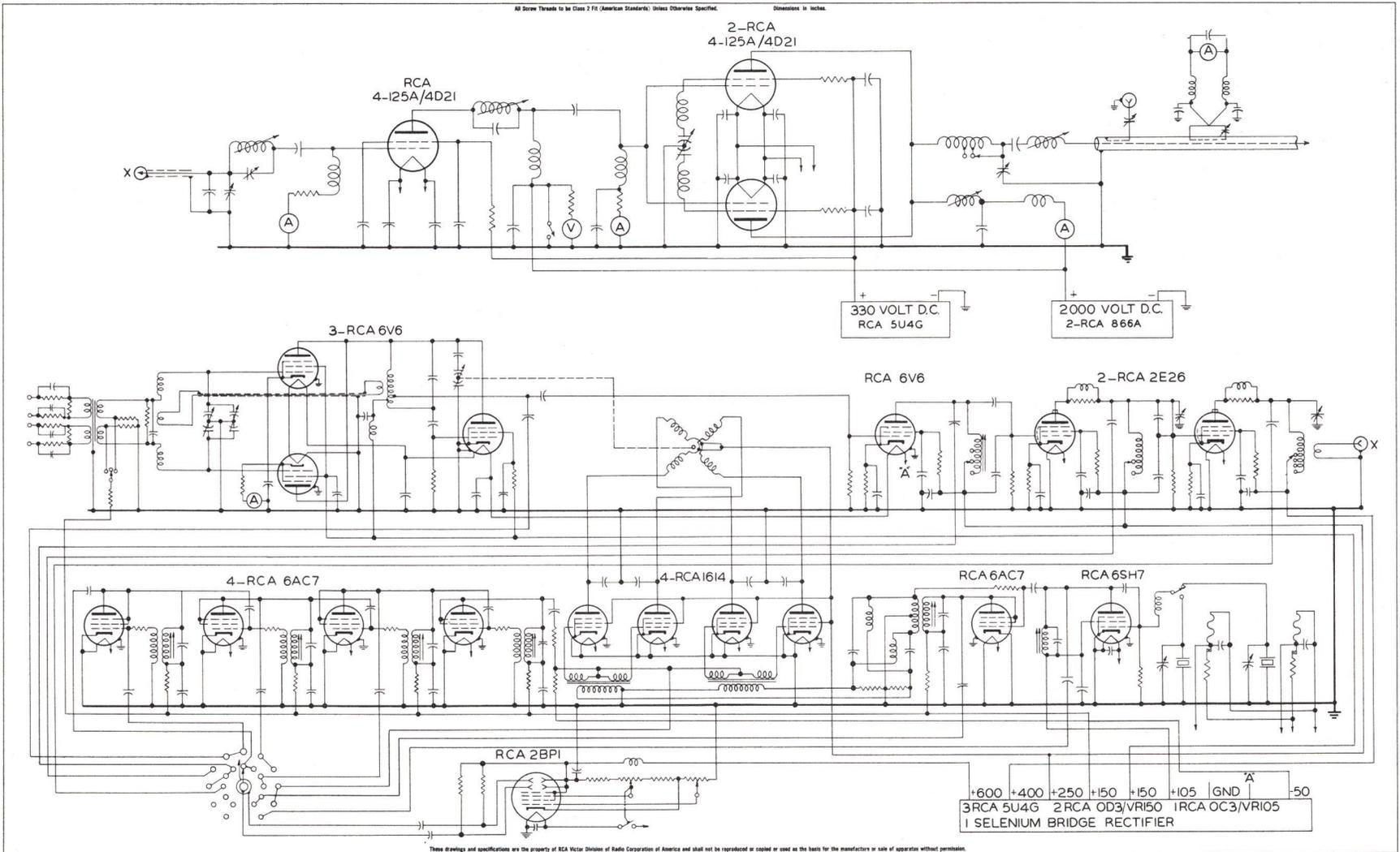
Figure 6-14 - TT-5004 Transmitter, Aural Portion, Schematic Diagram (T-618383)
