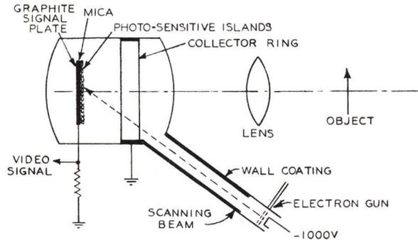
Figure 3-63 - Iconoscope Pick-up Tube
