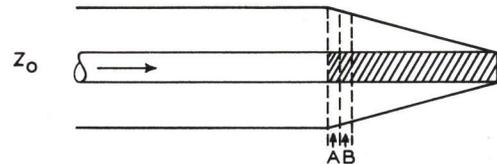
Figure 7-10 - Principle of R-F Load
