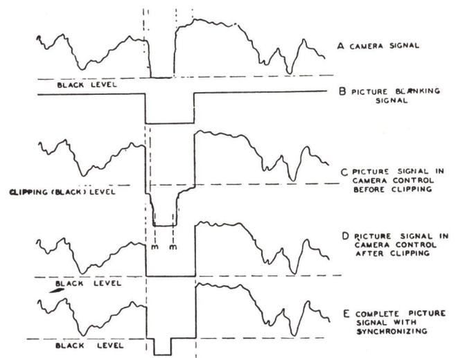
Figure 2-15 - Television Signal Wave Forms
