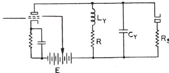
Figure 3-47 - Electronic Switch and Generator Circuit
