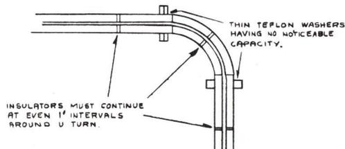
Figure 7-25 - Transmission Line Elbow Fitting
