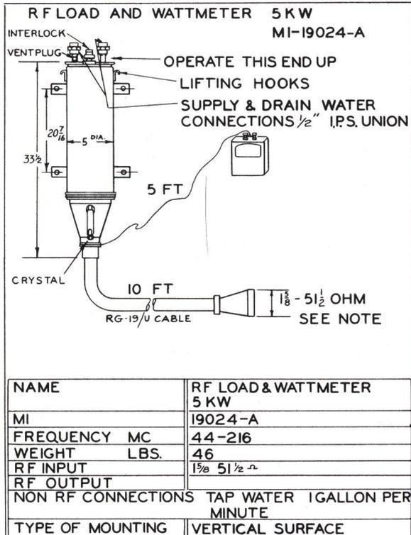
Figure 7-11 - R-F Load and Wattmeter Construction
