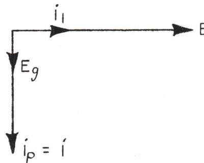
Figure 3-34 - Reactance Tube Circuit Vector Diagram
