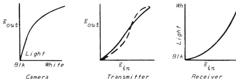
Figure 5-6 - Linearity Characteristics of TV System Elements
