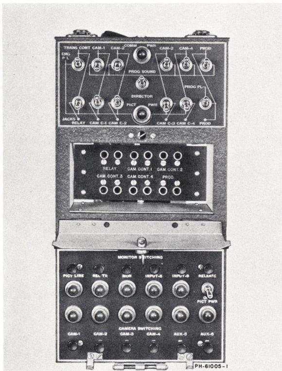
Figure 2-14 - Field Switching System, Front Side
