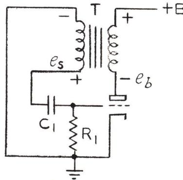
Figure 3-26 - Blocking Oscillator Circuit
