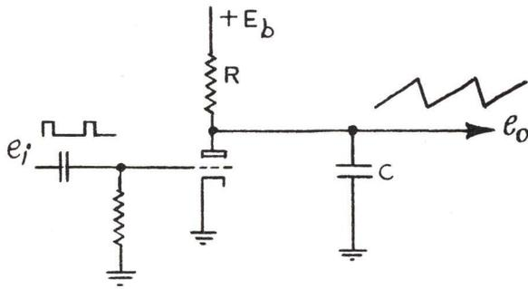
Figure 3-35 - Sawtooth Generator Circuit
