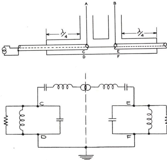
Figure 7-5 - Principle of Diplexer and Balun Units
