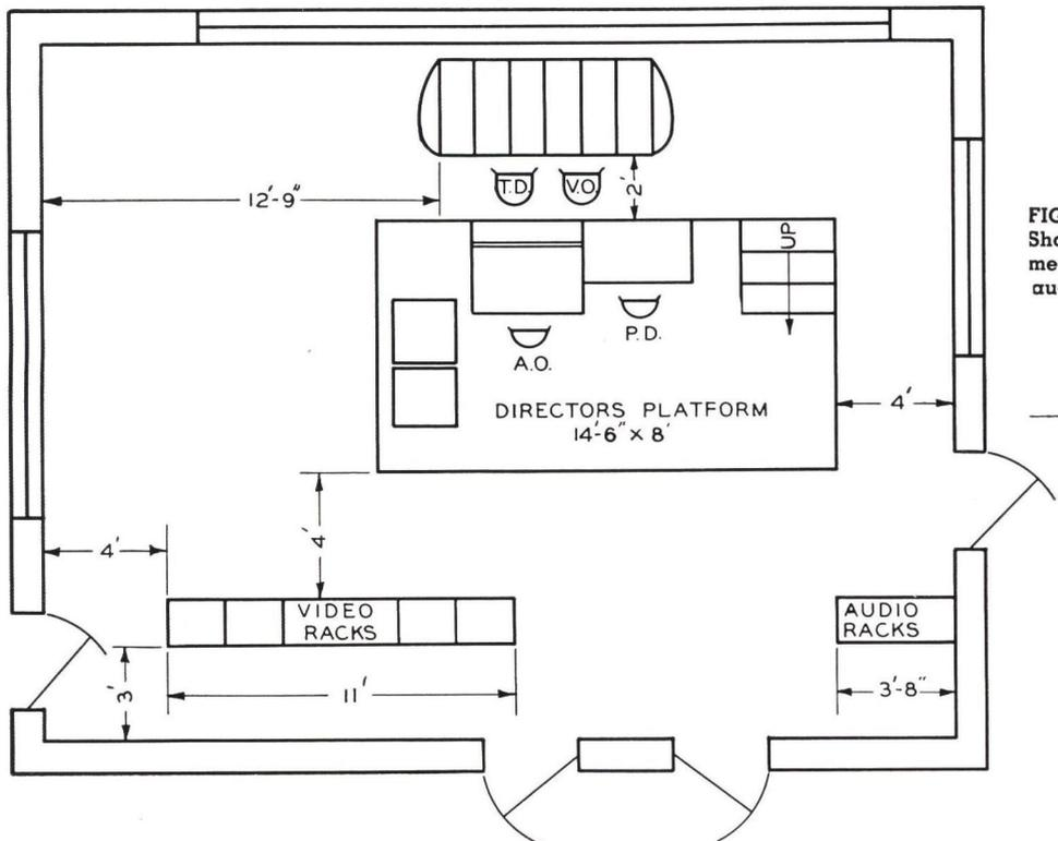
FIG. 23. Plan View of Type C Control Room Showing Program Director's Platform and Arrangement of Control Equipment. The racks contain audio and video amplifiers and power supplies.
