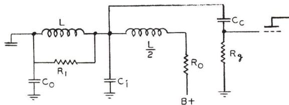
Figure 3-53 - Coupling Filter-connection
