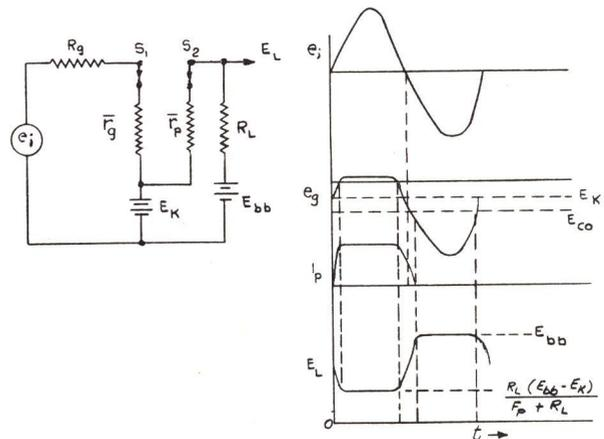
Figure 3-12 - Overdriven Amplifier, Equivalent Circuit and Wave Form.
