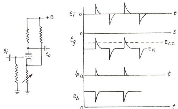
Figure 3-23 - Clipper Circuit
