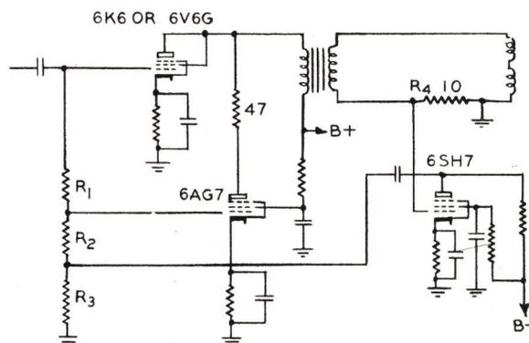
Figure 3-43 - Automatic Linearity Control Circuit
