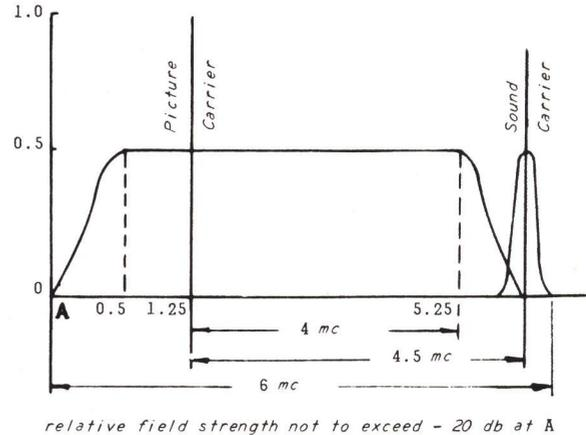
Figure 5-1 - Vestigial Sideband Amplitude Characteristic
