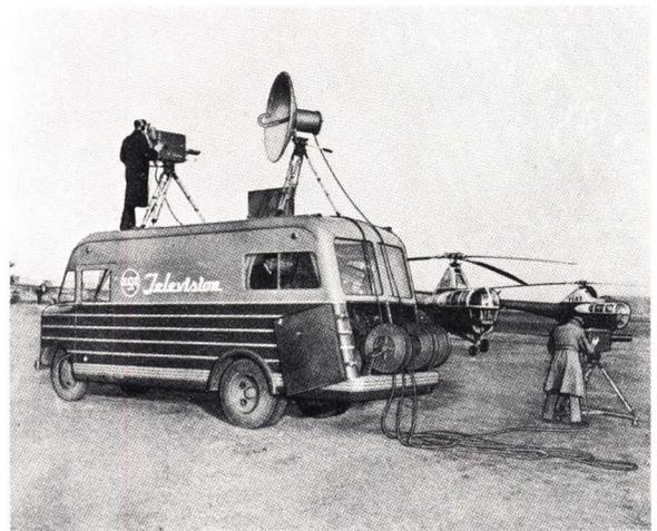
Figure 2-4 - Mobile Unit in Operation, with Camera and Relay Transmitter on the Roof
