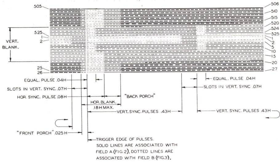
Figure 3-9 - Television Synchronizing Signal and Pulse Cross
