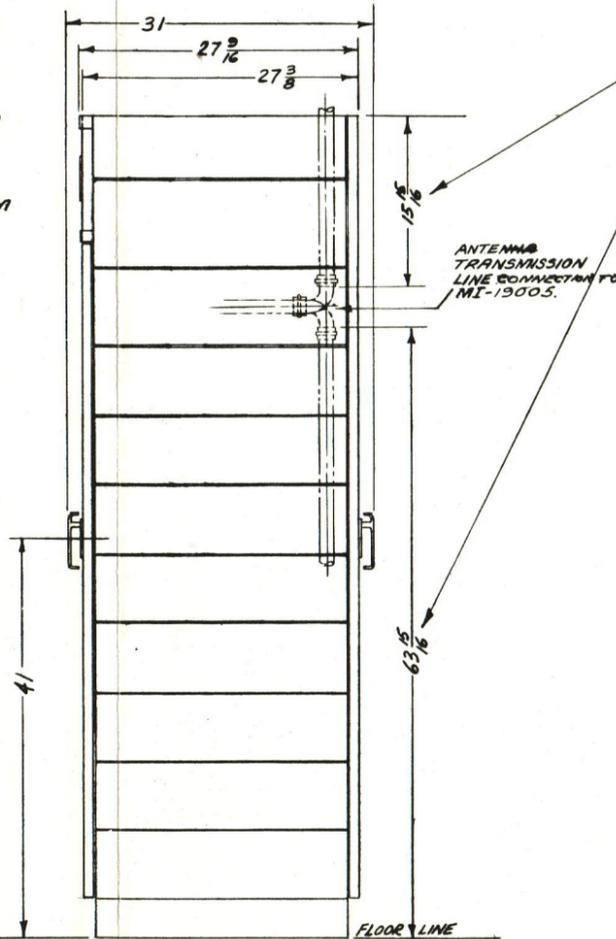
THESE DIMENSIONS INDICATE HOW FAR THE TRANSMISSION LINE MUST RUN INTO THE AURAL TRANSMITTER TO MAKE CONNECTION. THE VERTICAL TRANSMISSION LINE MAY BE INSERTED IN TO THE ELBOW FROM EITHER SIDE, TOP OR BOTTOM, AS SHOWN. THE LINE IS NOT FURNISHED WITH THE TRANSMITTER.
