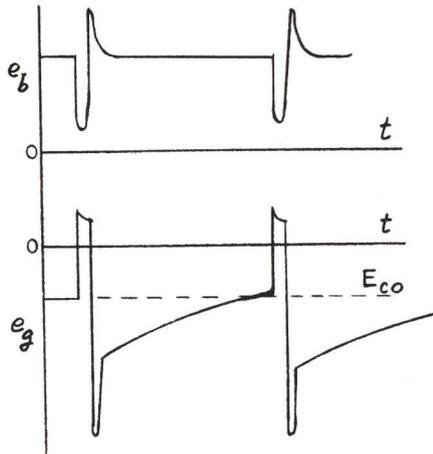
Figure 3-27 - Blocking Oscillator Operating Cycle
