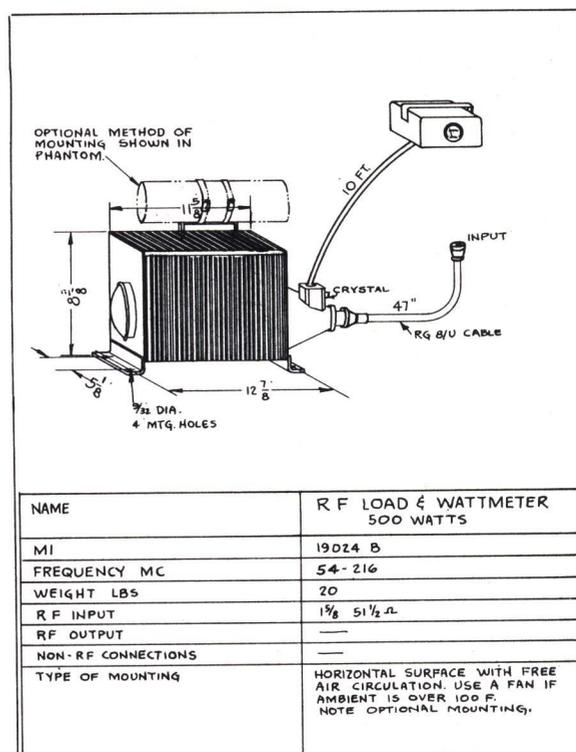
Figure 6-13 - 500-watt R-F Load and Wattmeter, MI-19024-B, Outling Drawing (M-450447)
