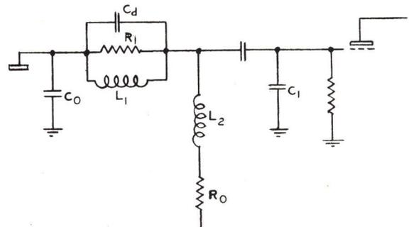
Figure 3-54 - Effect of Coil Capacity on Constant-K Filter
