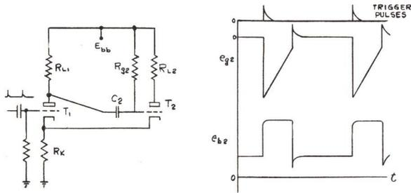
Figure 3-19 - "Flip-flop" Multivibrator
