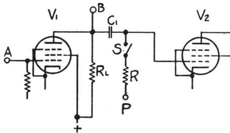
Figure 2-16 - Simplified Schematic Diagram of Clamp Circuit
