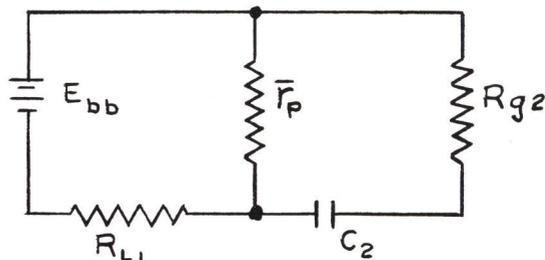
Figure 3-16 - Capacitor Discharge Circuit
