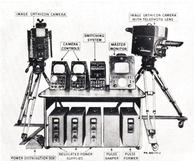
Figure 2-2 - Two-camera System Including Desk
