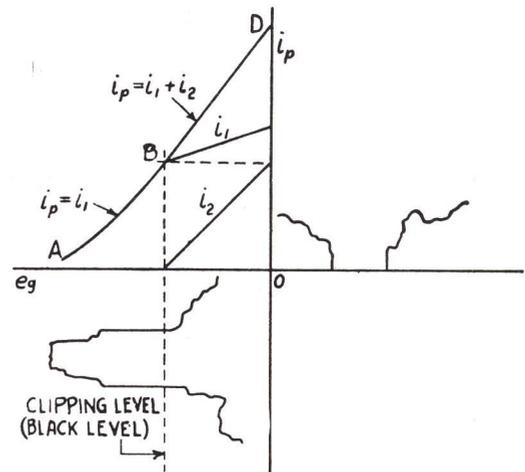
Figure 2-21 - Characteristic Curve of Linear Clipper
