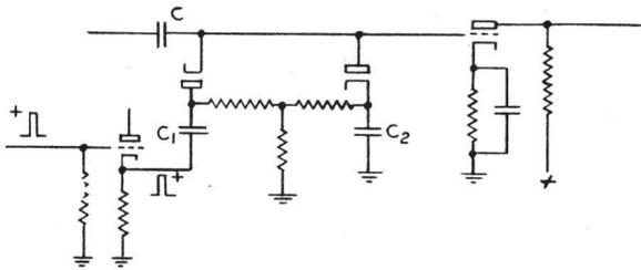
Figure 3-61 - Clamp Circuit for Single-polarity Keying Pulses
