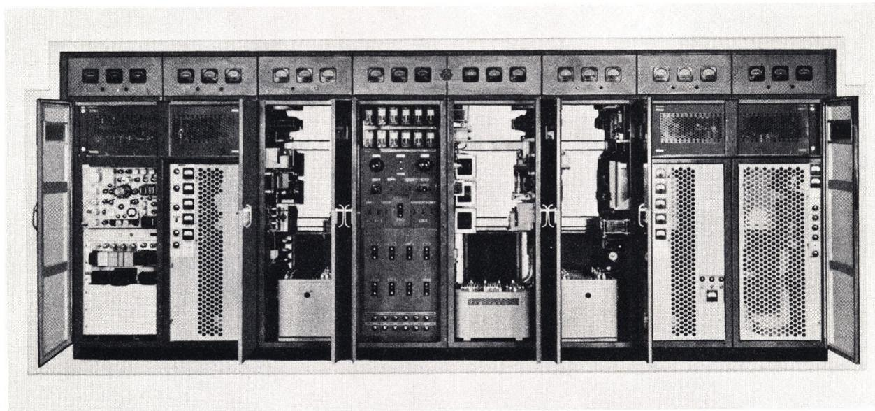
Figure 6-1 - TT-5A Television Transmitter, with front doors open to show accessibility. Frames 1 and 2 house the sound transmitter; frame 3, the sound-transmitter power supplies. Frame 4 is a centralized control panel for both sound and picture transmitters. Frames 5 and 6 contain the picture power supplies, while frames 7 and 8 house the picture transmitter. Each frame also has a full-length rear door, to give to each compartment maximum accessibility.
