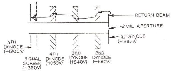
Figure 3-68 - Electron Multiplier for Image Orthicon
