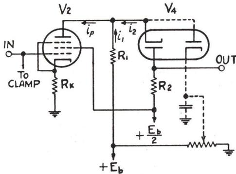
Figure 2-20 - Schematic Diagram of Linear Clipper
