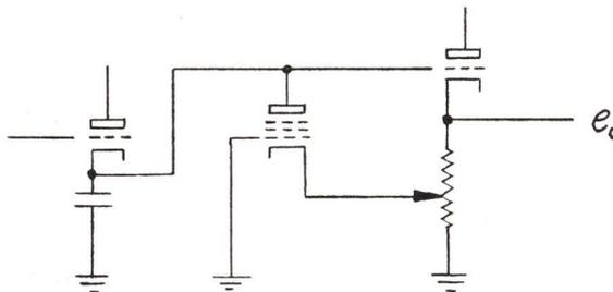
Figure 3-39 - Linearity Feedback Circuit
