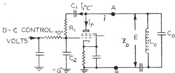
Figure 3-32 - Reactance Tube Circuit
