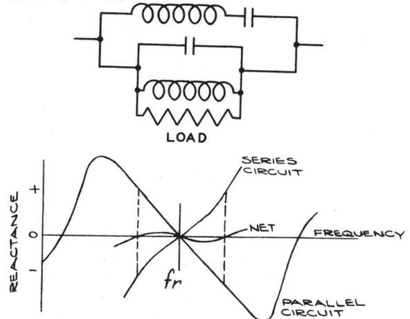
Figure 7-3 - Series-resonant and Parallel-resonant Circuit Combination
