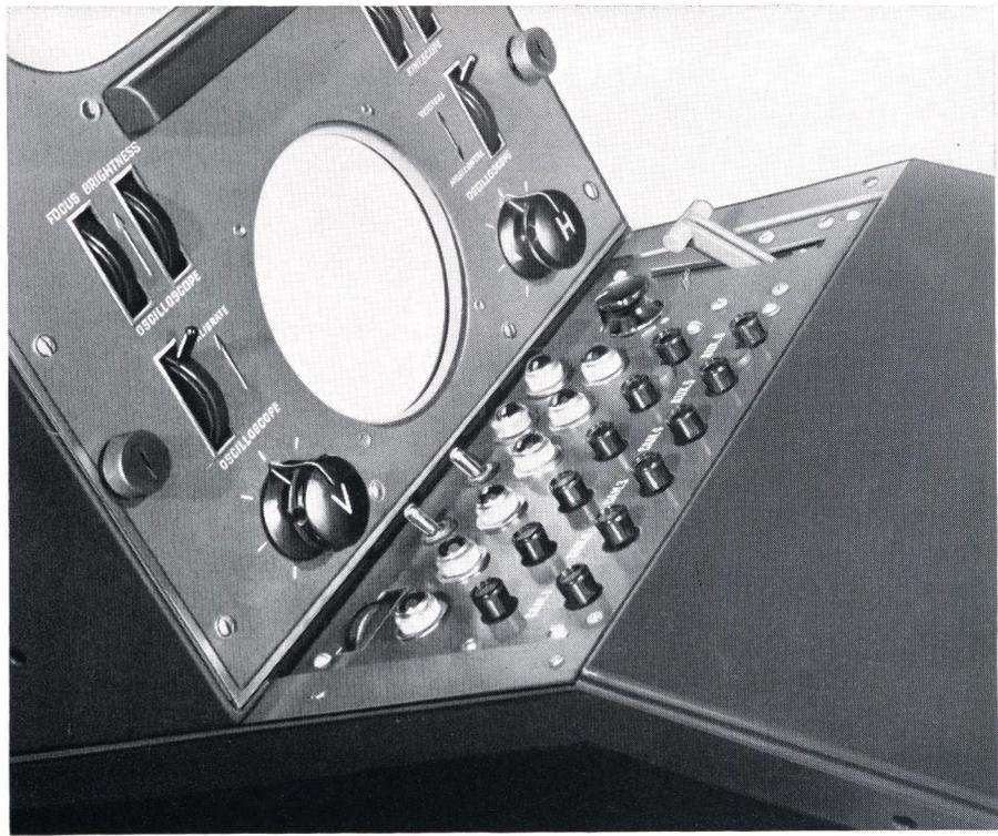
FIG. 17. (Above) Closeup of the TS-10A Switching System. With this system, the program director or the technical director can select the desired camera picture, or superimpose two pictures.
