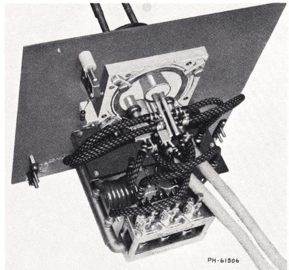
Figure 6-7 - Spare-tube Mounting Plate. With a spare tube mounted on this plate, and with most water connections made, the assembly is ready for quick insertion.
