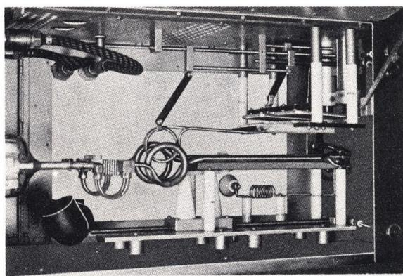
Figure 6-3 - Picture Power Amplifier, close-up view of the plate circuit. (The sound PA is identical, but reversed left-to-right.) Tuning is accomplished by flexible-shaft couplings to calibrated controls at the front. These controls are located behind the front doors, which on these frames are not interlocked.
