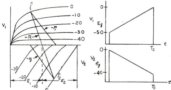
Figure 3-50 - Combined Characteristics of Beam Tetrode and Triode
