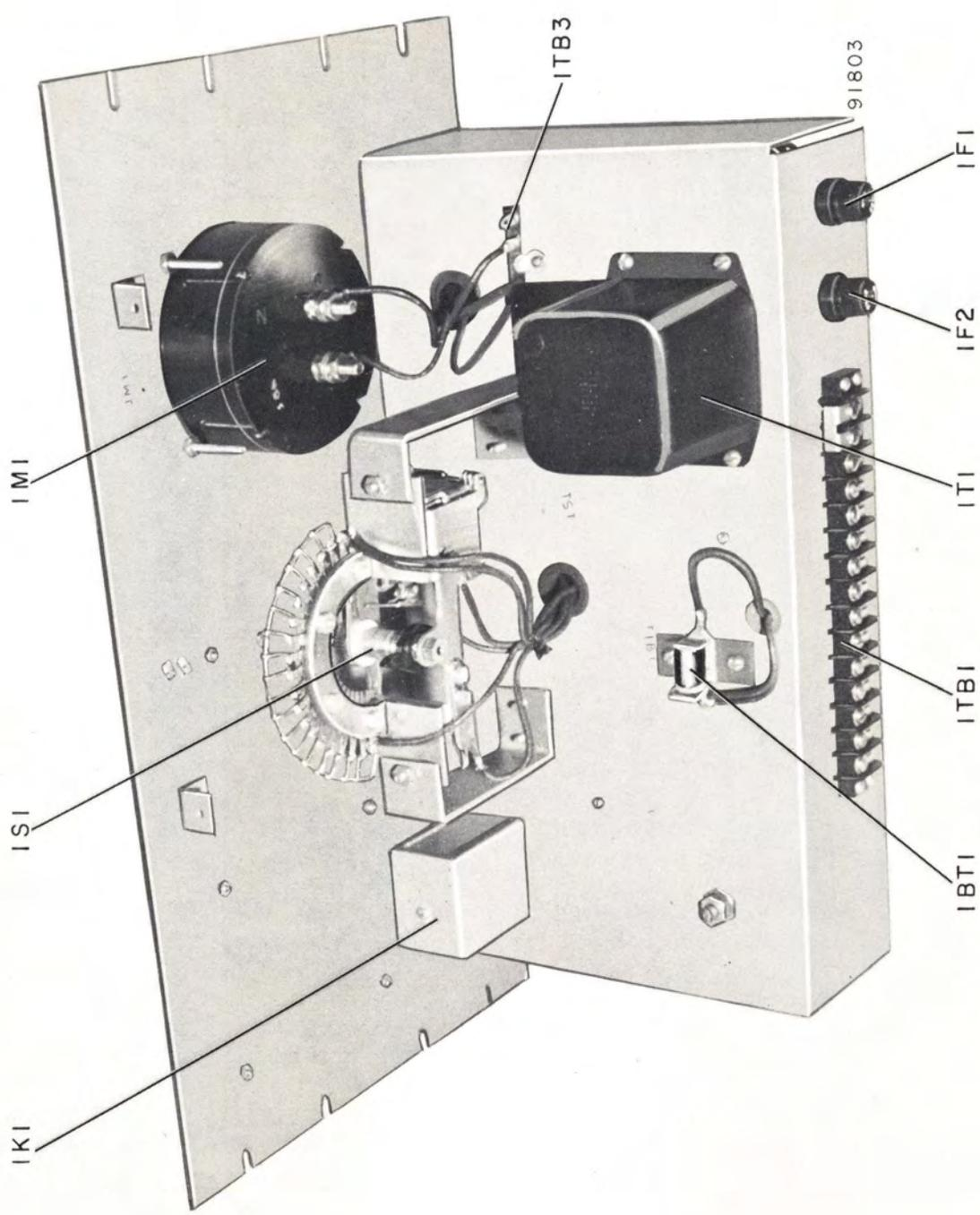
Figure 14 - Top View, BTR-20A Studio Control Unit
