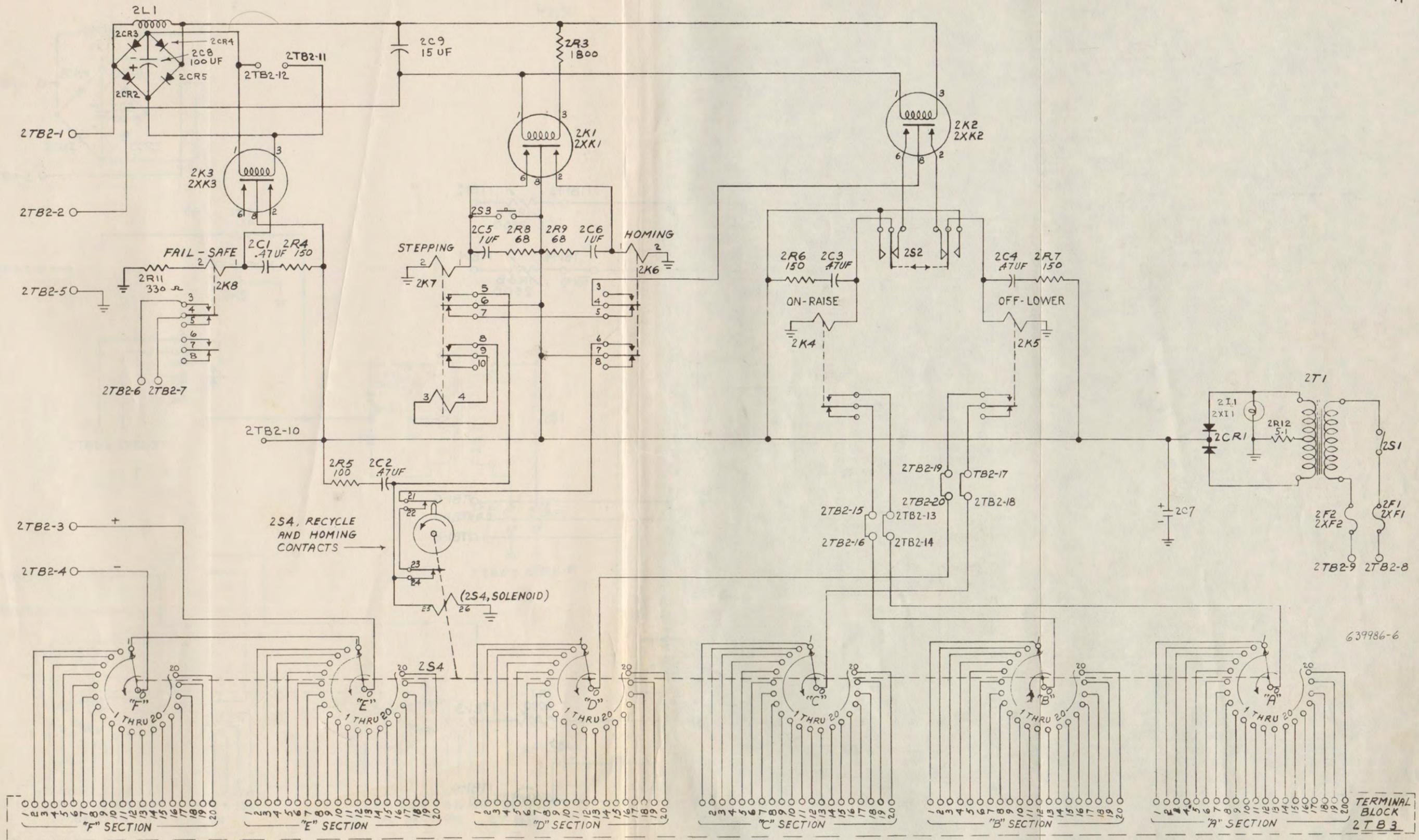
Figure 23 - Schematic Diagram, BTR-20A Transmitter Control Unit
