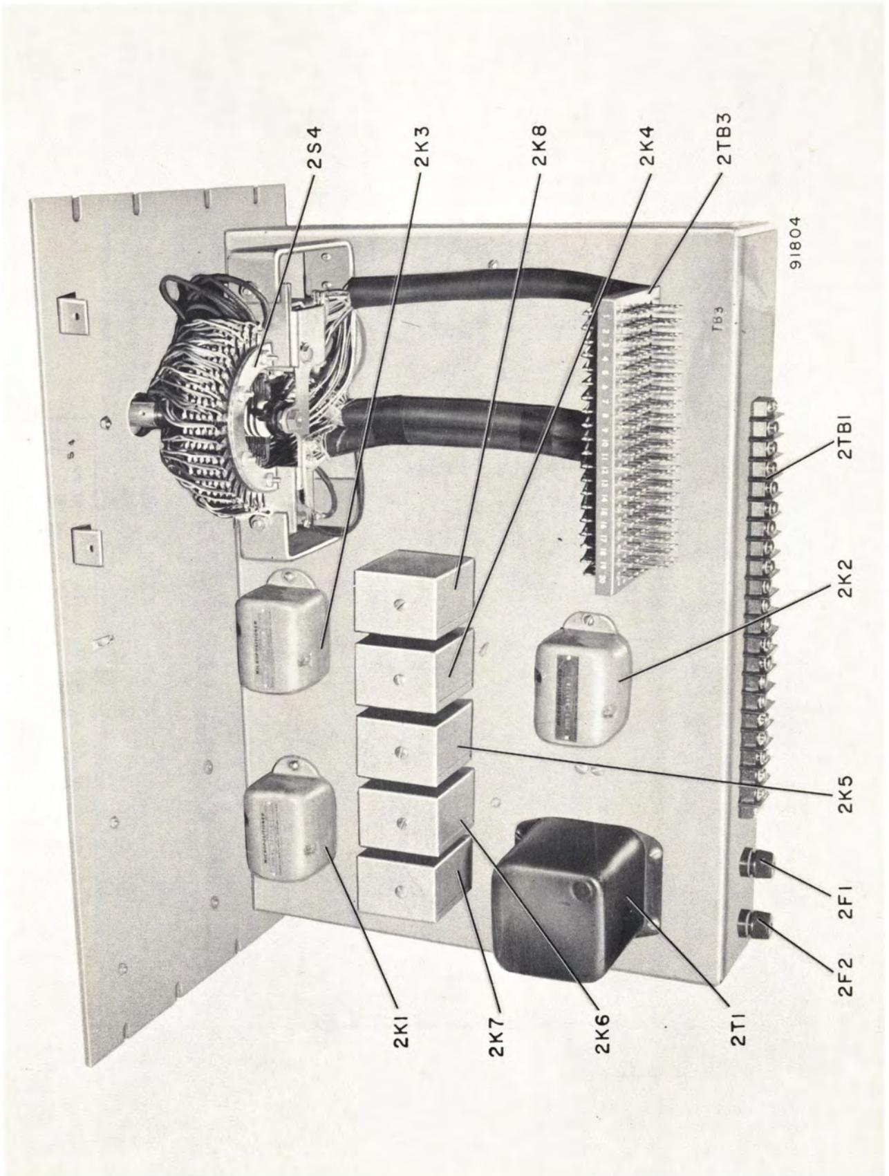
Figure 16 - Top View, BTR-20A Transmitter Control Unit
