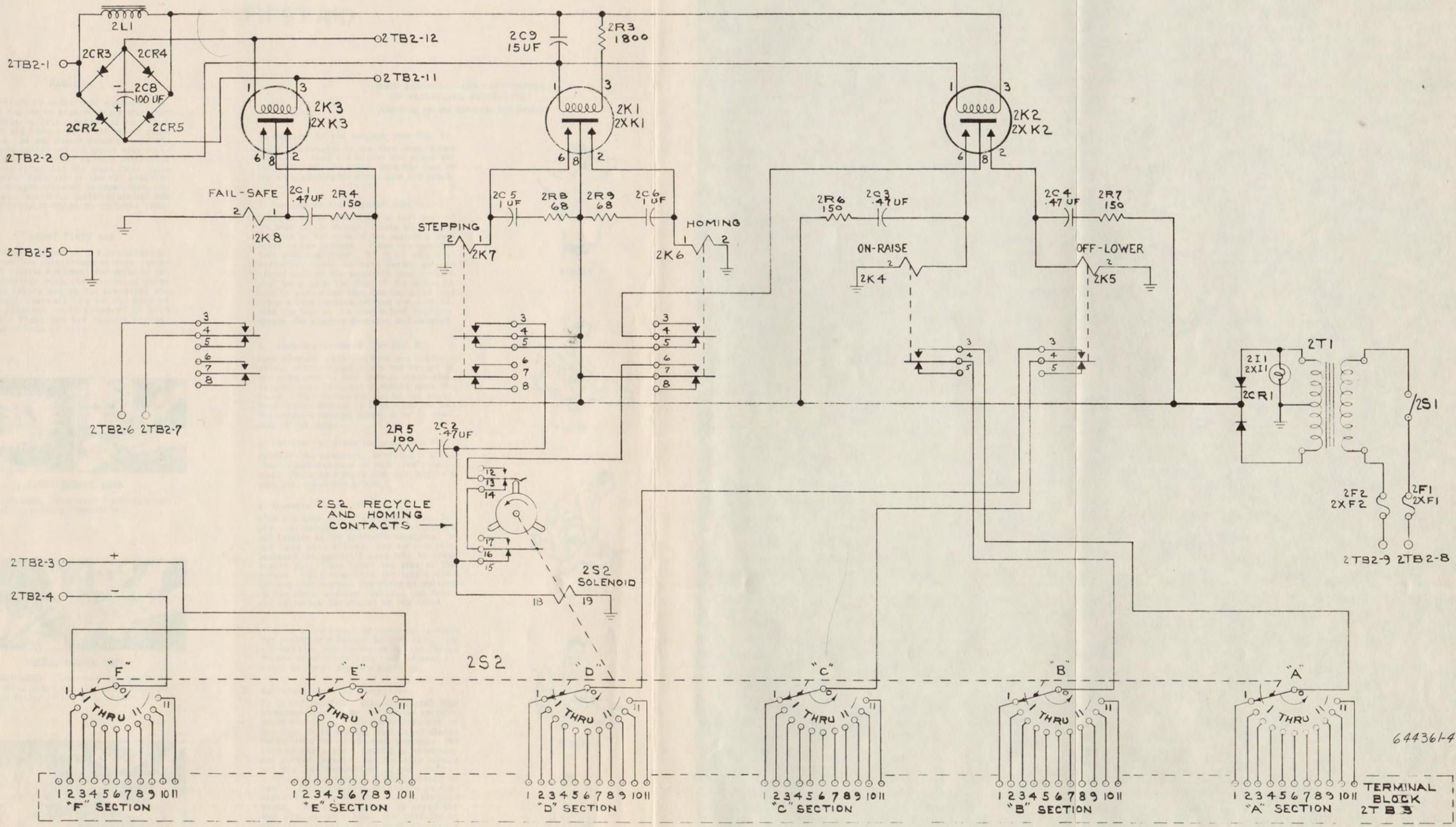
Figure 25 - Schematic Diagram, BTR-11A Transmitter Control Unit
