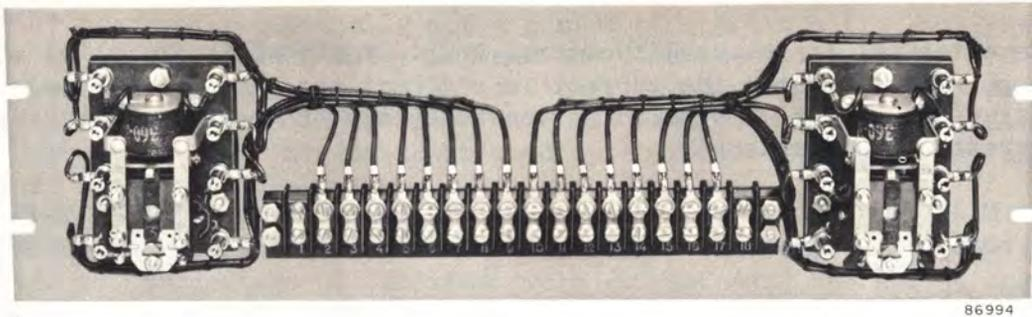
Figure 6 - Latching Relay Panel
