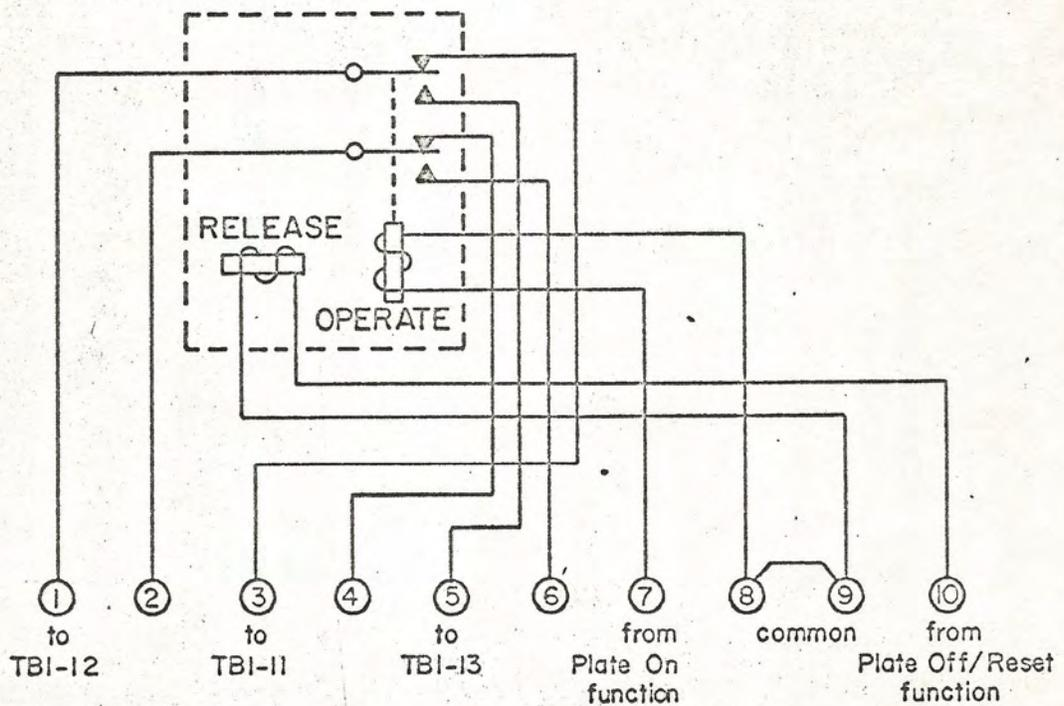
Figure 3. Latching Relay Unit - Rust Model 108-4A.
