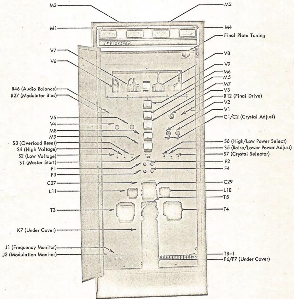
Figure 4. Front View of Bauer Model 707 Broadcast Transmitter.
