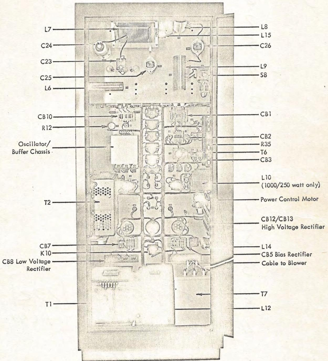
Figure 5. Rear View of Bauer Model 707 Broadcast Transmitter.
