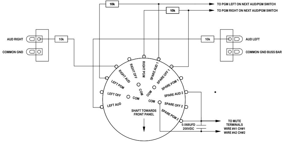
CHANNEL 3 & 4 AUD/PGM SWITCH WIRING
