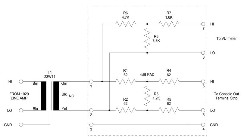
T1 - T2 Primary, 60 ohm Secondary, 600 ohm -1dB, 20Hz TO 20KHz at +24dBM
