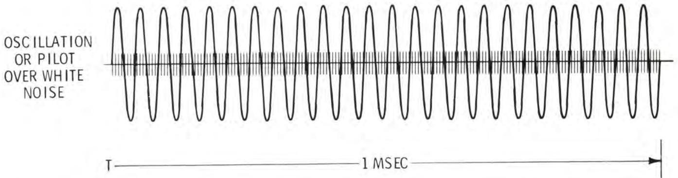
If the noise is a high frequency oscillation, the scope sweep can be adjusted to lock in on the signal. White noise is random in nature and can not be "synced".
