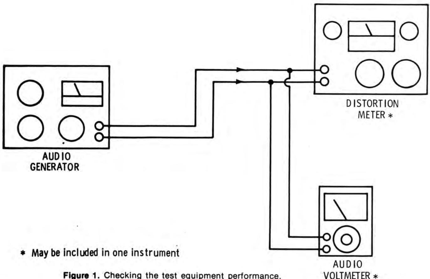
Figure 1. Checking the test equipment performance.
