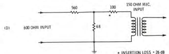
A simple method of resistive coupling to the mic. input.
