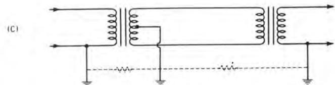
Multiple ground connections open the door for "ground loops" that could render the measurements invalid.
