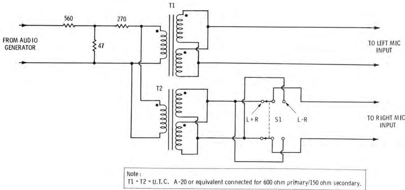
Figure 4E. A coupling unit for stereo tests.
