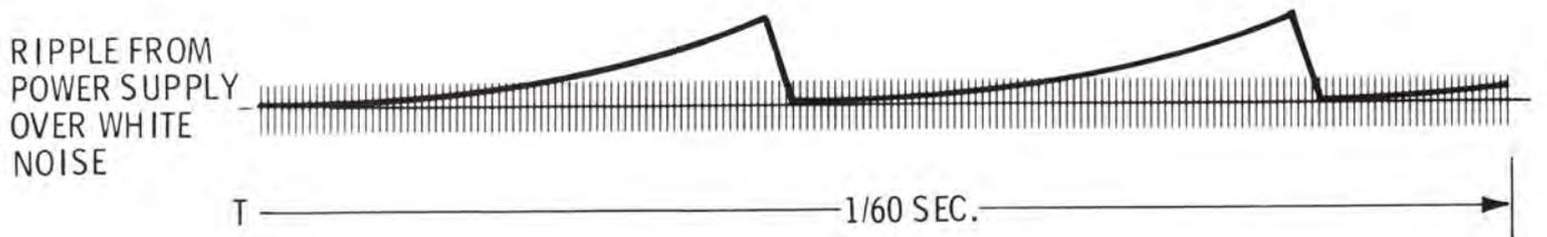
This type of noise will also sync. to the line but it's frequency will be a multiple of the power line frequency.
