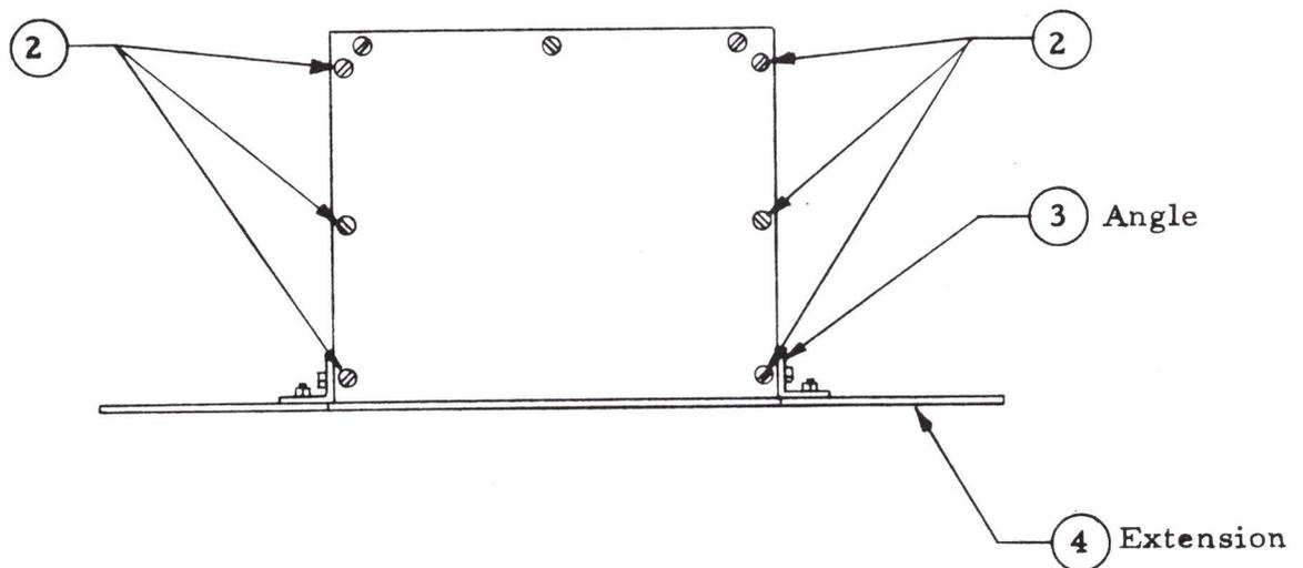
1. Loosen the four Phillips screws on the front panel approximately 1/2 turn.
