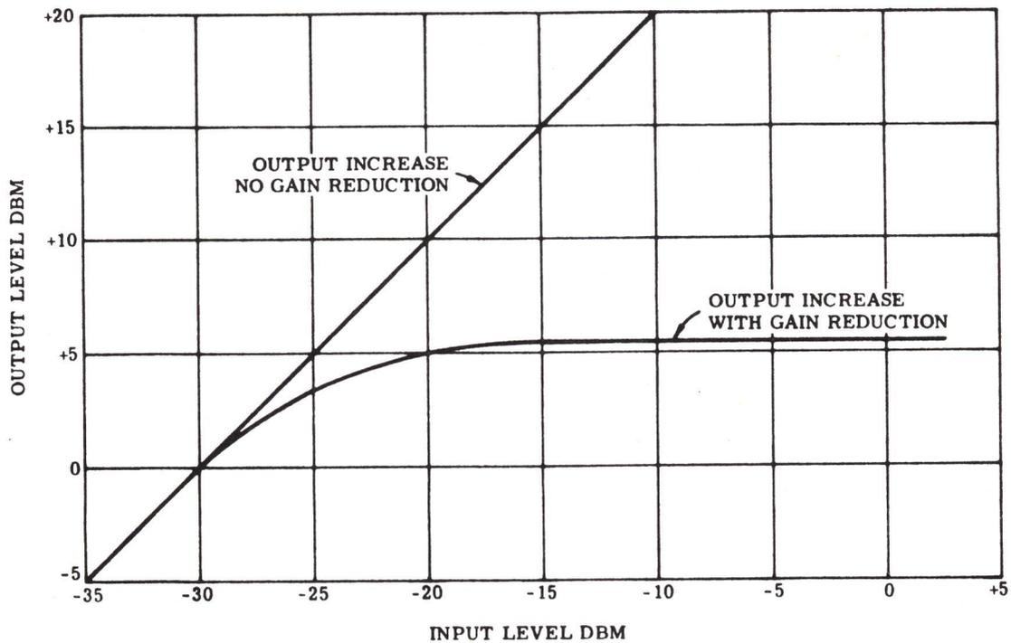
FIGURE 1. TYPICAL GAIN REDUCTION PLOT FOR LA-3A
