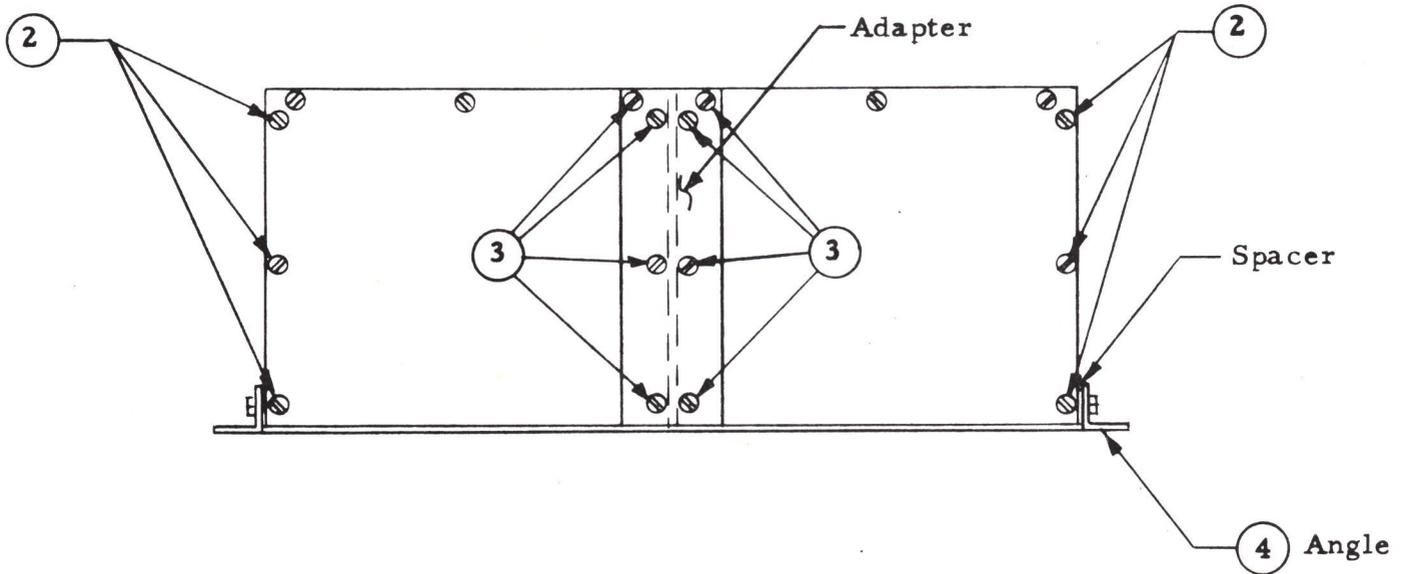
1. Loosen the four Phillips screws on the front panel of each unit approximately 1/2 turn.
